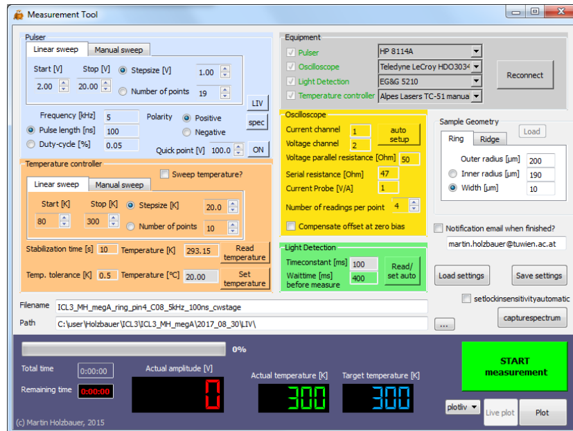
Fig. 2.39: Graphical user interface of the self-developed Python program used to control and automate the measurement process.
