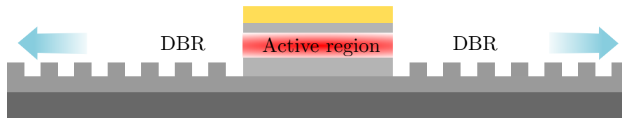
Fig. 2.22: Illustration of a lateral distributed-Bragg reflector grating.
