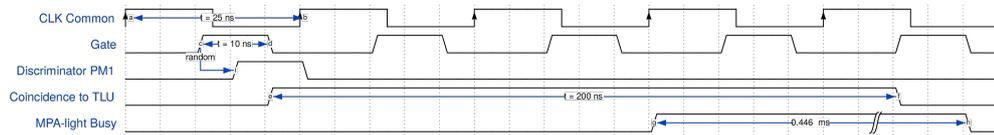
Figure 10.4: The timing of signals important for the trigger gating and busy logic used throughout the test beam. CLK refers to the 40 MHz clock. The coincidence to **TLU** signal is used with the coincidence of three other PMs to provide the trigger.
