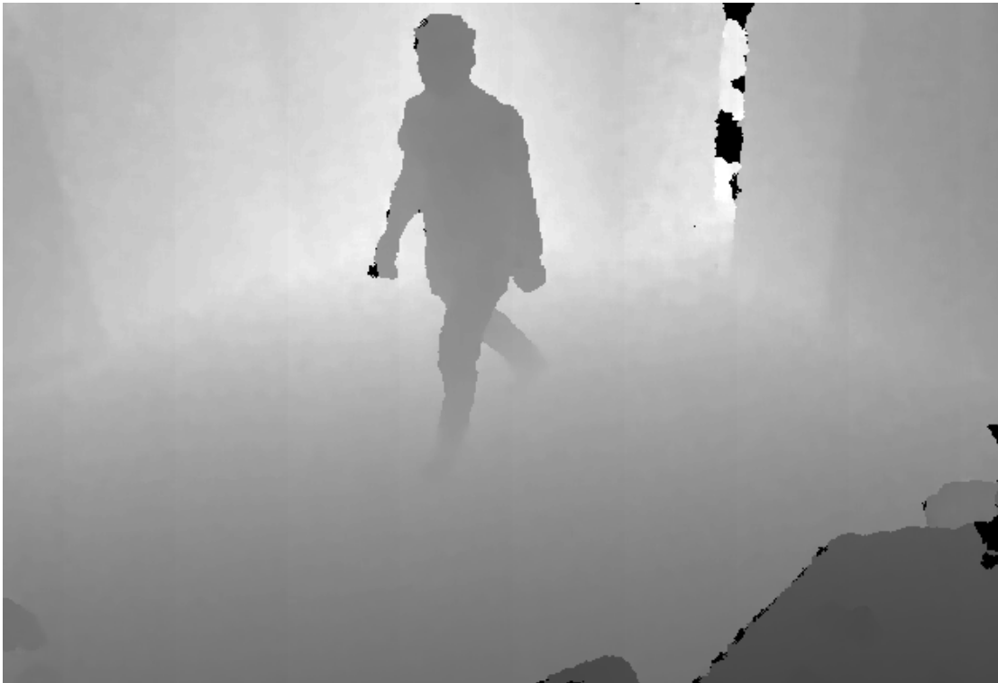
Figure 1.2: Visualization of depth information obtained from a 3D sensor as gray values: the closer the object the darker the representation. The person’s face is not visible.
