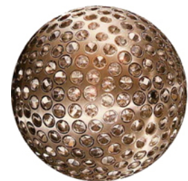
Figure 3: LAGEOS 1 - SLR Satellite with a diameter of 60 cm and 426 reflectors. Source: NASA
