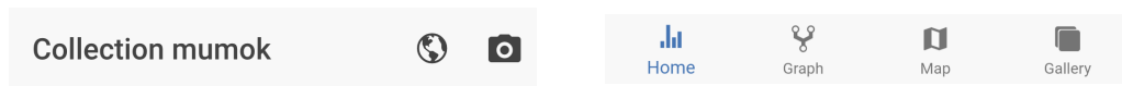
Figure 4.4: Top toolbar bar with the buttons to change the language and scan a tag (left) and bottom navigation bar
