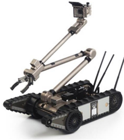
Fig. 3. 2 Military robot: iRobot PackBot (iRobot, 2014)
