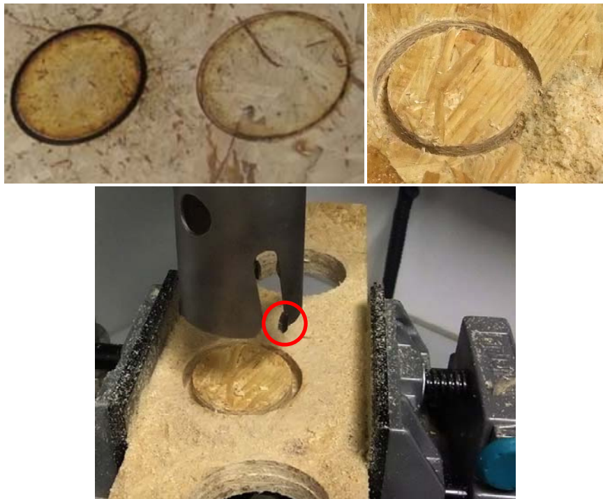
Figure 44. Influence of the thermal load during cutting out samples for the \mu CTE. Above from left to right: bi-metal hole saw without cooling intervals, bi-metal hole saw with cooling intervals, hard metal hole cutter without cooling intervals. Below: HM Mehrzweck-Lochsäge Bohrkronen Wolfcraft 3782000 \varnothing 45
