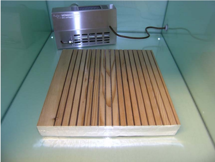
Figure 11. Scheme for VOC testing of an acoustic plate in a 225 l testing chamber with one emitting surface left unsealed
