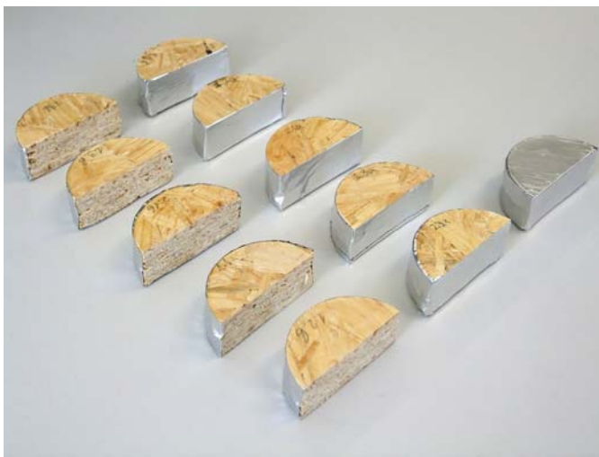
Figure 40. Experimental setup for examination of the edge effects on VOC emissions
