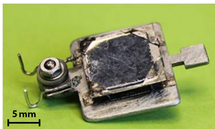
Fig. 2.14. The polycrystalline Rh foil is mounted to the sample plate. The type K thermocouple wires (NiCr/Ni) are attached to the Rh foil and two isolated contact electrodes.
