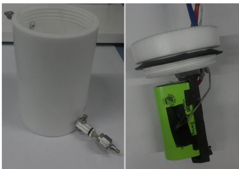
Figure D5. Picture of the PTFE gas sampling cell. Left: Cell body. Right: Lid with attached cell and thermocouple.
