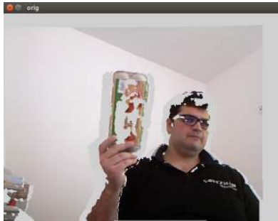
Figure 8.1: Original 3D view of the camera. Grey pixels are denoting areas without 3D information.
