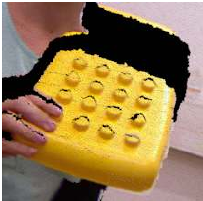
Figure 5.2: Part of a 3D-Image, where we can see that the contour of the yellow object is not accurate.
