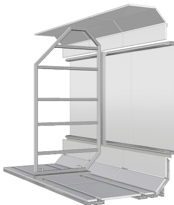
5.6 Frame attached to profiles
