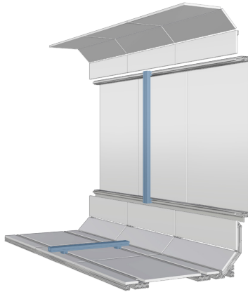
5.5 Pre-mounted profiles connecting pairs of rails
