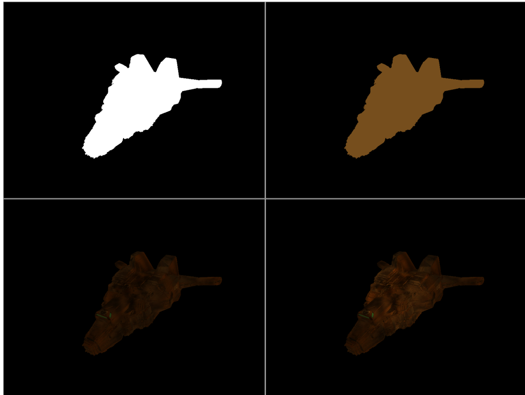
Figure 2.7: Examples of pixel shaders: the same model a.) without any shaders, b.) with a uniform color, c.) with a texture and d.) a shader rendering a spotlight onto it.
