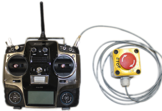
Figure 2.10: Picture of the emergency switch connected to the Handset via a cable to allow instant use.
