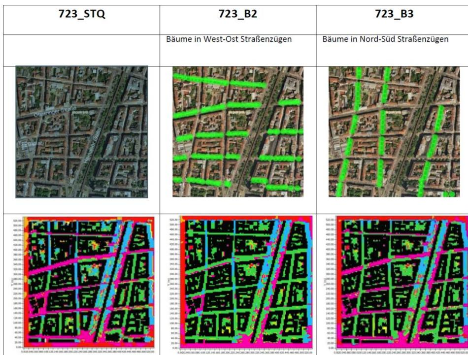
Figure 25: Simulation of planning measures of the Urban Fabric Types project in one quadrant. Top: city structure and planned measures (trees on the streets). Bottom: urban climate effects (source: Stiles et al. 2014, 7–10).
