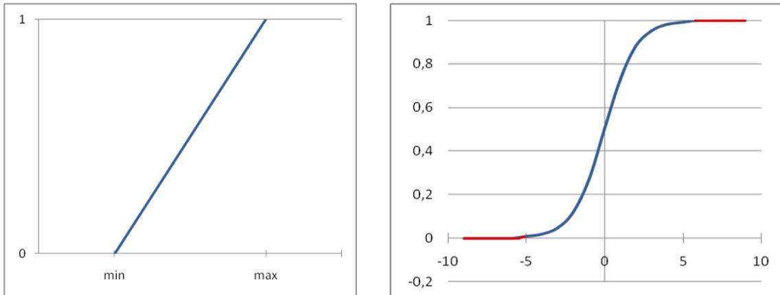
**Figure 7: Distribution functions of fuzzy membership.** Left: Linear distribution of the values from 0 to 1 where 0 is the minimum value and 1 the maximum value. Right: Example of a S-shaped distribution (source: own illustration).
