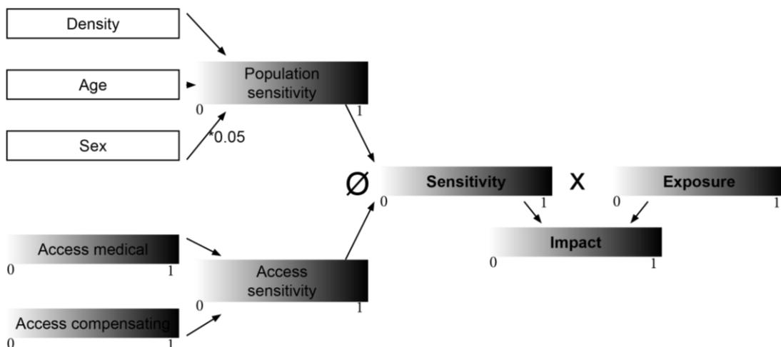
Figure 9: Flow chart showing the combination of indicators to calculate the impact (own illustration).
