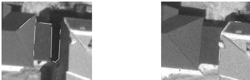
Figure 7.5: Two images for the reconstruction of a small garage between two larger buildings with the extracted image edges from pyramid level 3 ( 120 \mu\text{m} ) superimposed to them in white colour (example 2). The garage could not be reconstructed correctly because one of its roof edges was occluded in all images but the right one in the figure, where it could not be extracted due to the low contrast.
