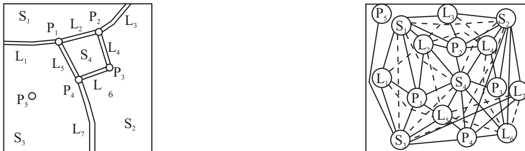
Figure 5.8: Left: the results of classification: Point regions P_i , edge regions L_i , homogeneous regions S_i , and their borders. Right: the corresponding feature adjacency graph. The full lines describe direct neighbourhood relations, the broken lines indirect ones. According to [Fuchs, 1998].
