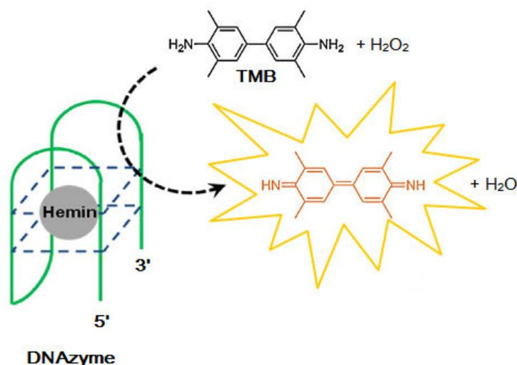
**Figure 1.5.4:** Schematic illustration of a DNAzyme-based calorimetric assay with TMB as substrate.
