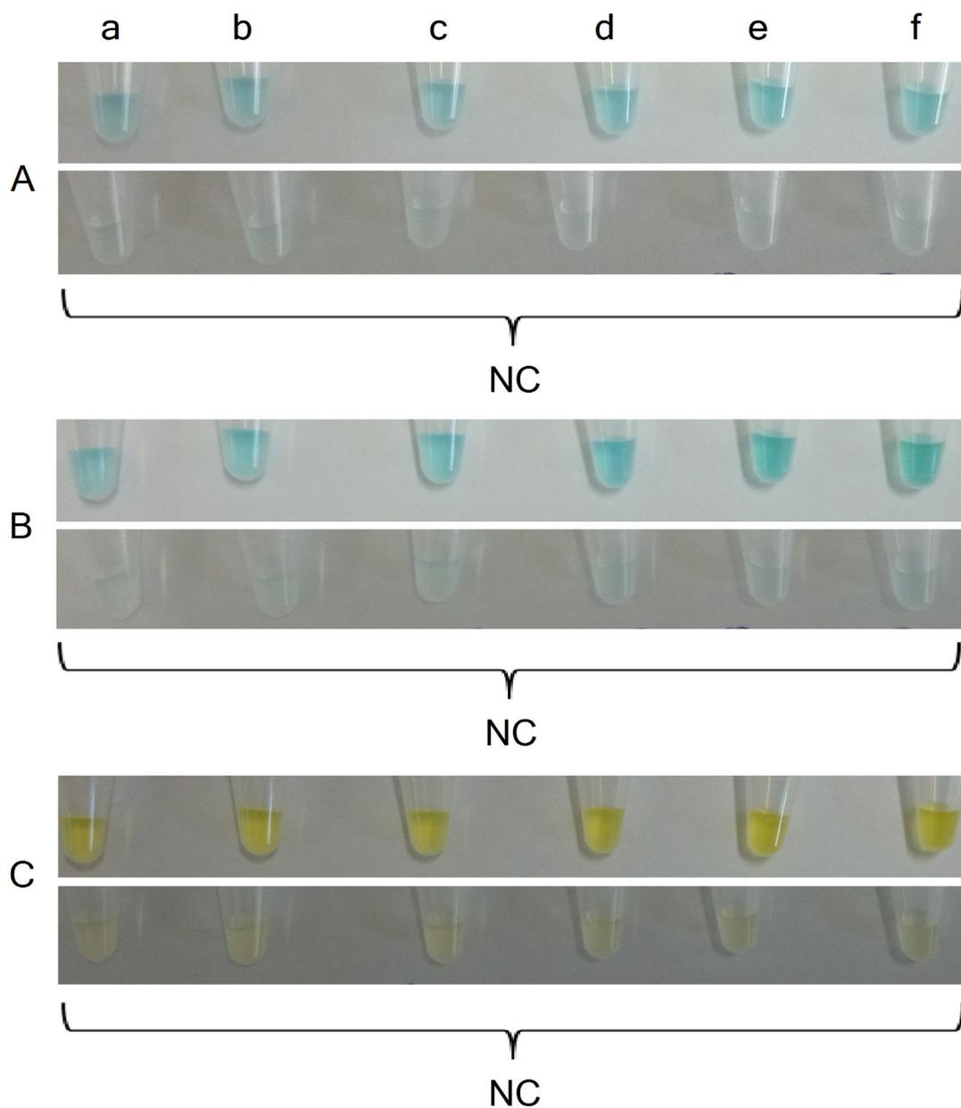
**Figure 4.1.8:** Different percentages of acetonitrile (a-f) in the reaction solution. Photographs of H<sub>2</sub>O<sub>2</sub>-mediated oxidation of TMB using different percentages of acetonitrile (a-f, Tab. 4.1.15) in the reaction solution after (A) 10- minutes and (B) 20- minutes incubation and (C) stopping the reaction after 20 minutes by addition of H<sub>2</sub>SO<sub>4</sub>. Negative controls without DNAzyme are shown below the respective samples.
