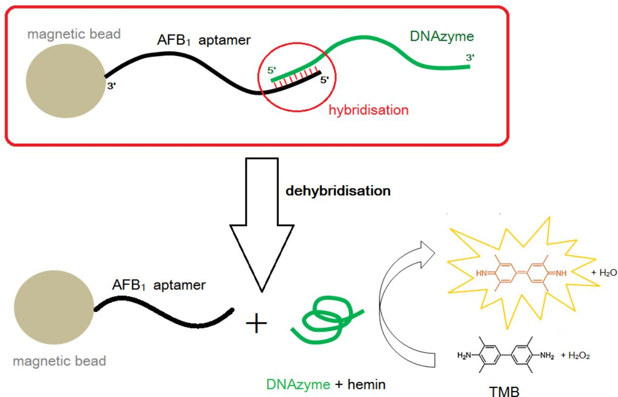
**Figure 4.2.1:** Schematic illustration of the dehybridisation experiments.
