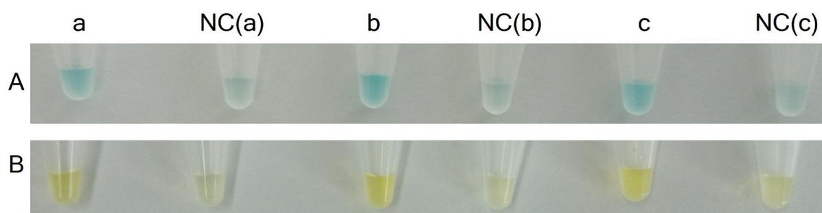
**Figure 4.2.3:** Different concentrations of hybrid used for immobilisation onto the beads. Photographs of H<sub>2</sub>O<sub>2</sub>-mediated oxidation of TMB of samples with different concentrations of immobilised hybrid [(a) 10  $\mu$ M, (b) 20  $\mu$ M and (c) 40  $\mu$ M] after (A) 30- minutes incubation and (B) stopping the reaction after 30 minutes by addition of H<sub>2</sub>SO<sub>4</sub>. Respective negative controls [NC(a), NC(b) and NC(c)] are shown next to the samples.
