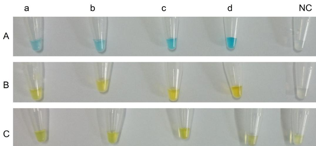
**Figure 4.1.4:** Different concentrations of TMB in the substrate solution. Photographs of oxidation of different concentrations of TMB (a-d, Tab. 4.1.5) in the substrate solution after (A) 20- minutes incubation, after (B) stopping the reaction after 20 min by addition of H<sub>2</sub>SO<sub>4</sub> and (C) seven hours after stopping the reaction.
