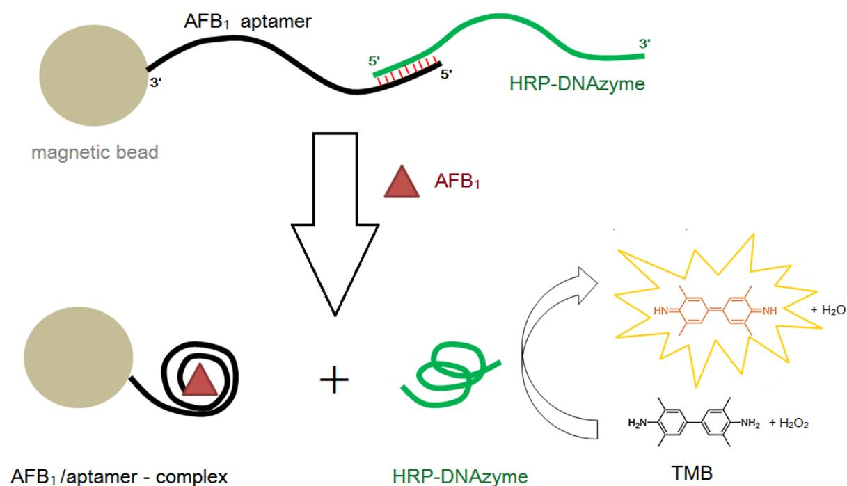
**Figure 2.1.1:** Schematic illustration of the planned aptamer- and DNAzyme-based detection of AFB<sub>1</sub>.
