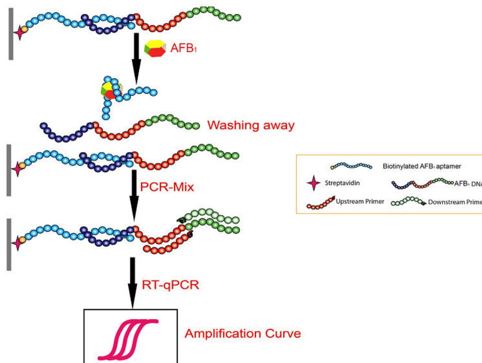
**Figure 1.4.1:** Schematic illustration of the aptasensor for the detection of AFB<sub>1</sub> [4].
