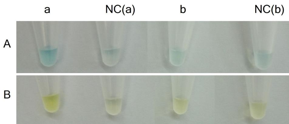
**Figure 4.2.2:** Different washing buffers used for beads with immobilised hybrid. Photographs of  $\text{H}_2\text{O}_2$ -mediated oxidation of TMB of samples with different washing buffers used for the beads with immobilised hybrid (a and b, Tab. 4.2.1) after (A) 30- minutes incubation and (B) stopping the reaction after 30 minutes by addition of  $\text{H}_2\text{SO}_4$ . Respective negative controls [NC(a) and NC(b)] are shown next to the samples.
