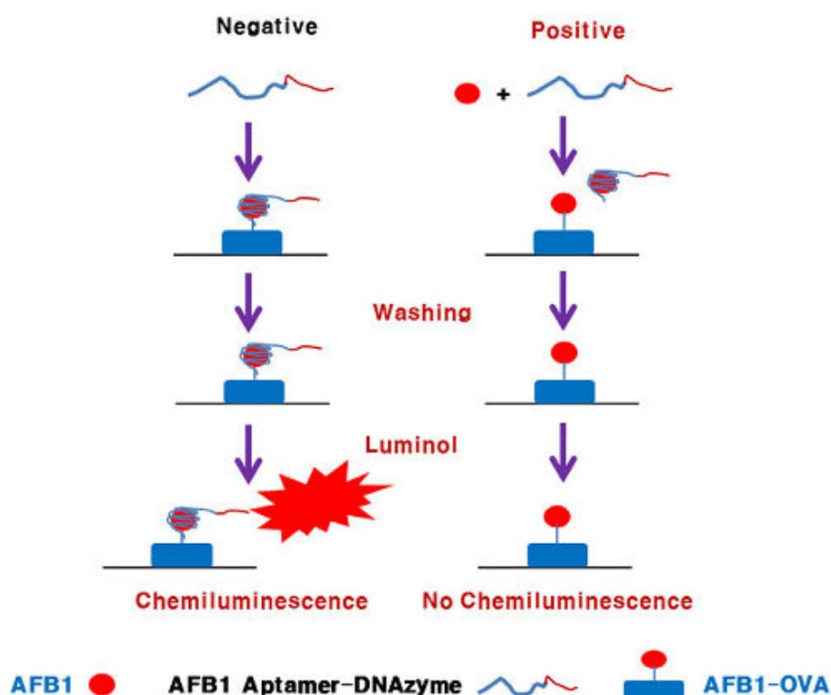
**Figure 1.4.2:** Schematic illustration of the chemiluminescence competitive aptamer assay for the detection of AFB<sub>1</sub> [6].
