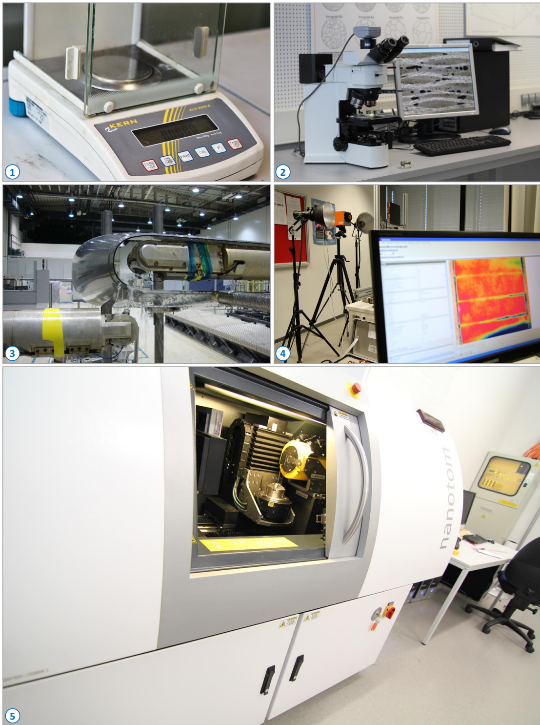
❖ Figure 1.4 — Destructive and non-destructive testing methods for porosity determination: (1) Acid digestion. (2) Materialography. (3) Ultrasonic testing. (4) Active thermography. (5) 3D X-ray Computed Tomography (GE Phoenix|xray nanotom XCT system at the University of Applied Sciences Upper Austria - Wels Campus).
