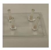
Figure 17.: Assembled blank chip with adhesive tape and polymer tubes to ensure microfluidic flow for cell adhesion measurement.
