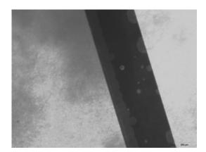
Figure 40.: Electrode delamination due to chlorpromazine. This issue not only resulted in a failure of impedance measurement but also lead to cell death.
