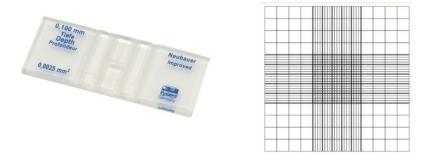
Figure 15.: Neubauer chamber for cell counting, performed under the microscope.
