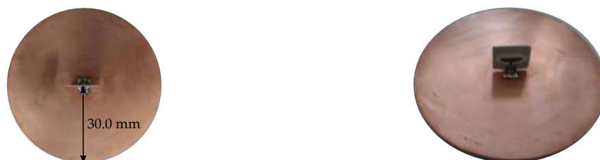
Figure 3.8: Adding a ground plane to the plane-symmetrical self-complementary antenna will diminish the cable currents. This technique is a tradeoff between accurate measurements and small form factor. The ground plane is realized out of a 0.2 mm RO4003C substrate. The stubs on the top were not removed.
