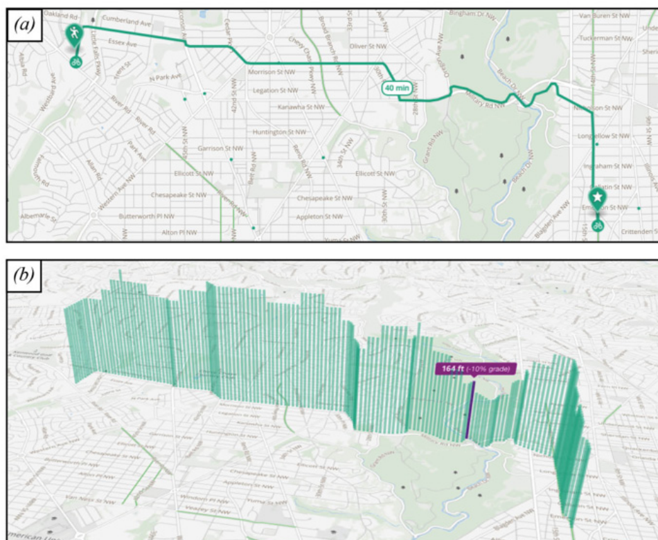
Figure 3-16 The conceptual route planning interface developed by MapBox for the Washington Bike Share scheme, featuring (a) the 2D route planner, and (b) the interactive 3D elevation profile for the route shown in (a). (Liu, 2015).
