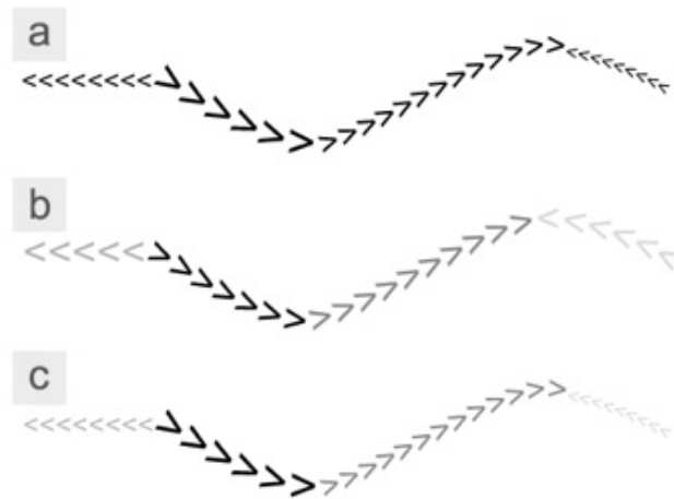
Figure 3-13 Some possibilities for arrow symbolisation. Arrows indicate downward slope direction, with steepness encoded by: (a) arrow size, (b) colour saturation, and (c) arrow size and colour saturation. Based on the work of Huffman (2009).
