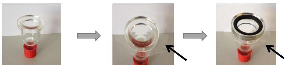
Figure D-15 Attachment of the PDMS Membrane (see black arrows) between the reaction chambers
