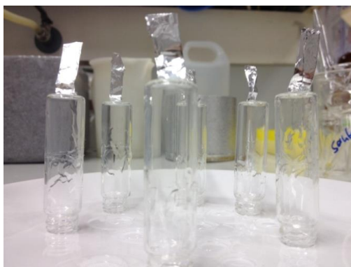
Figure D-12 PDMS coated vials holding an aluminium foil attachment for later removal from the glass mould
