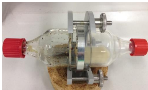
Figure D-14 Novel membrane reactor
