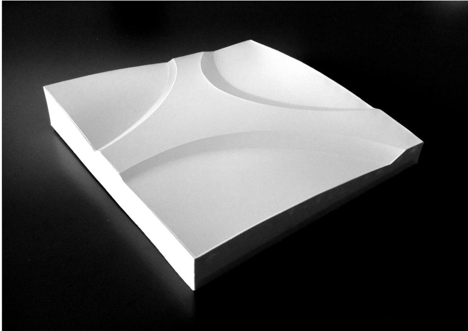
Figure 6.9: final model made out of paper and polypropylene
