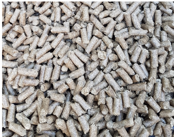
Figure 3.3: Produced fuel pellets of the fuel mixture Chicken Litter High (CLH)
