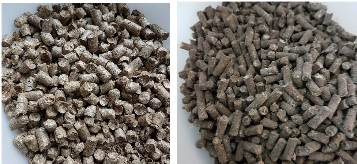
Figure 3.1: Pre-pelletized raw materials straw (left) and chicken litter (right)
