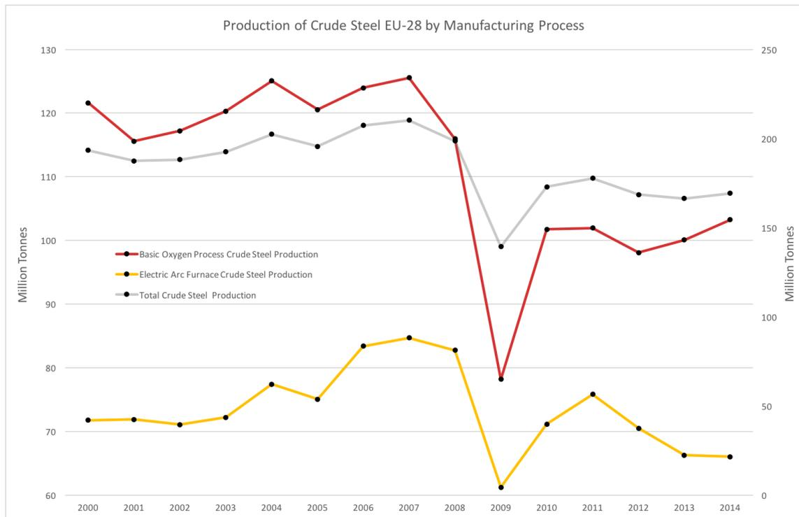
Figure 5: Production of Crude Steel EU-28 by Manufacturing Process, Data: World Steel Association.
