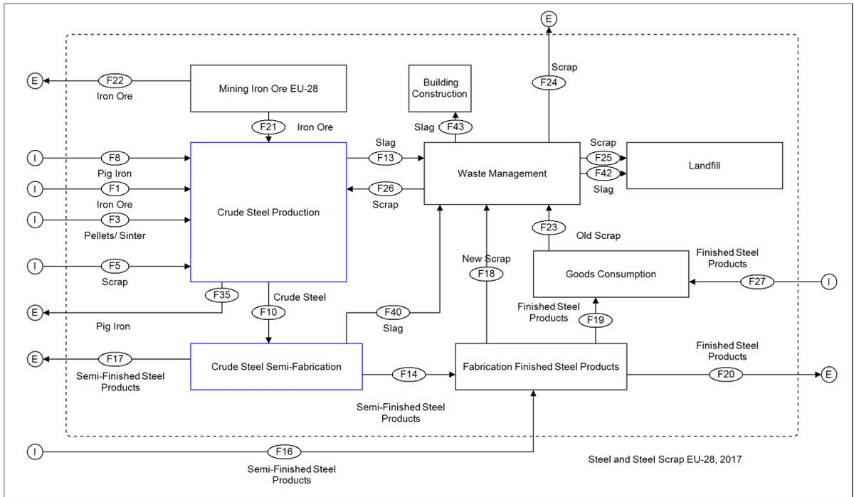
Figure 9: Steel Production and Scrap Flows EU-28, Illustration based on various sources.
