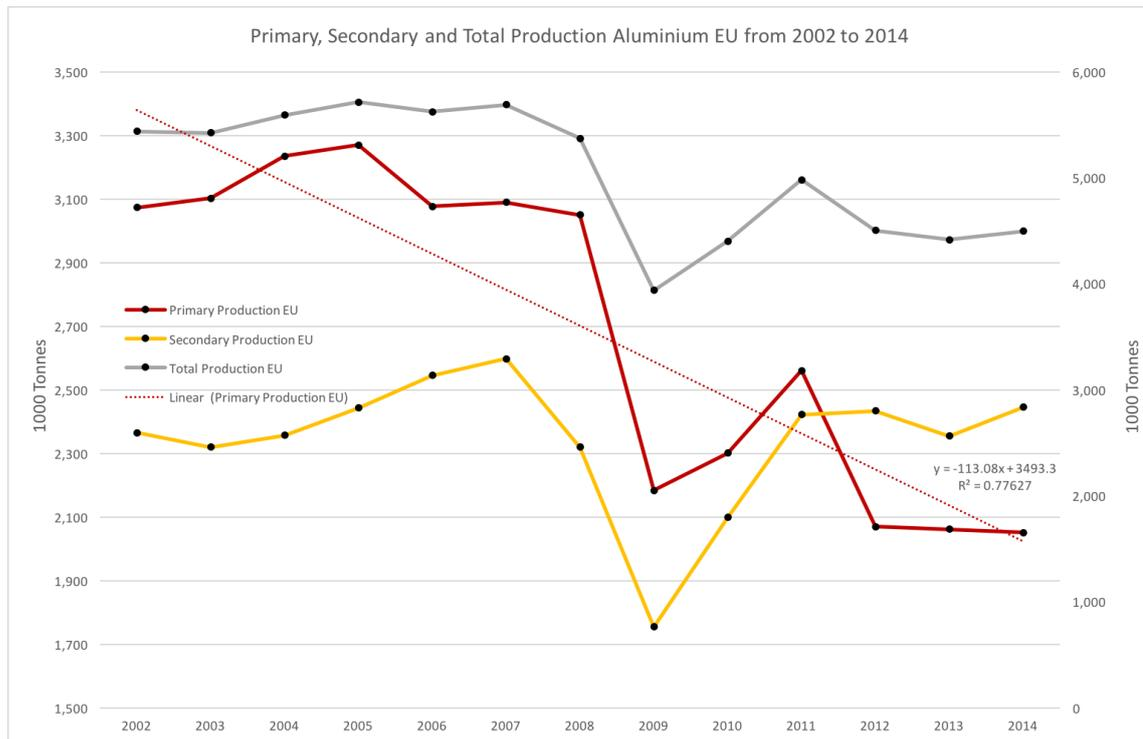
Figure 17: Primary, Secondary and Total Production Aluminium EU from 2002 to 2014, Data: European Aluminium.
