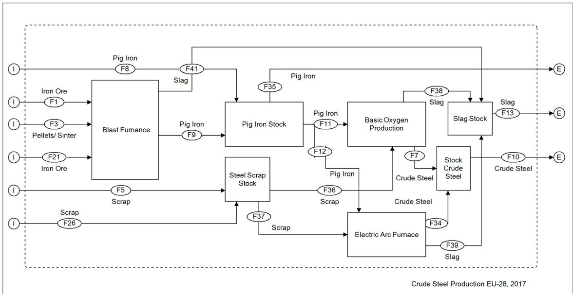
Figure 10: Sub-process Crude Steel Production, Illustration based on various sources.
