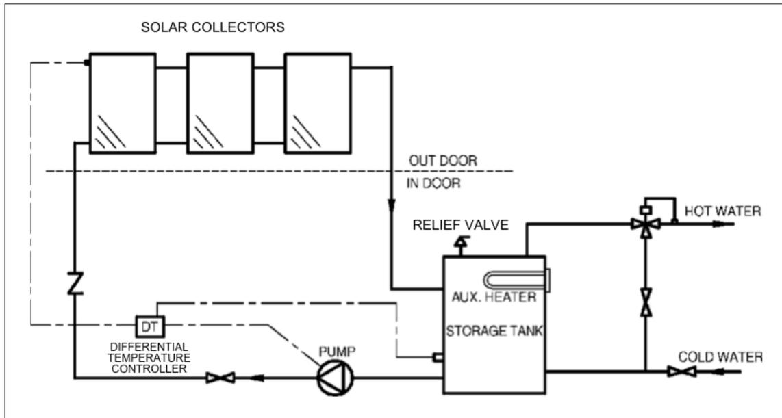
**Figure 25:** Direct circulation system. *Source:* Kalogirou 2009, 265.
