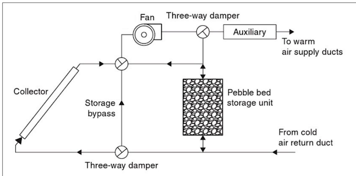
**Figure 24:** Basic solar air heating system with pebble bed storage. *Source:* Kalogirou 2009, 351.
