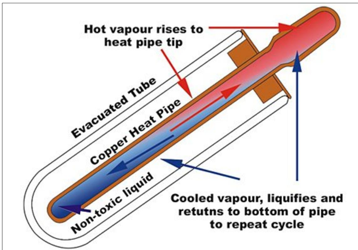
**Figure 22:** Evaporating-condensing cycle in the heat pipe of an evacuated tube collector. *Source:* China Senior Supplier, available from: [http://www.chinaseniorsupplier.com/Energy/Solar\\_Energy\\_Products/1592425113/Pressurized\\_vacuum\\_tube\\_solar\\_collector\\_instal\\_on\\_the\\_wall.html](http://www.chinaseniorsupplier.com/Energy/Solar_Energy_Products/1592425113/Pressurized_vacuum_tube_solar_collector_instal_on_the_wall.html)
