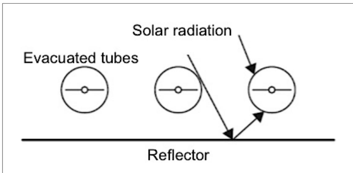
**Figure 23:** Evacuated tube collectors with reflector. *Source:* Kalogirou 2009, 134.
