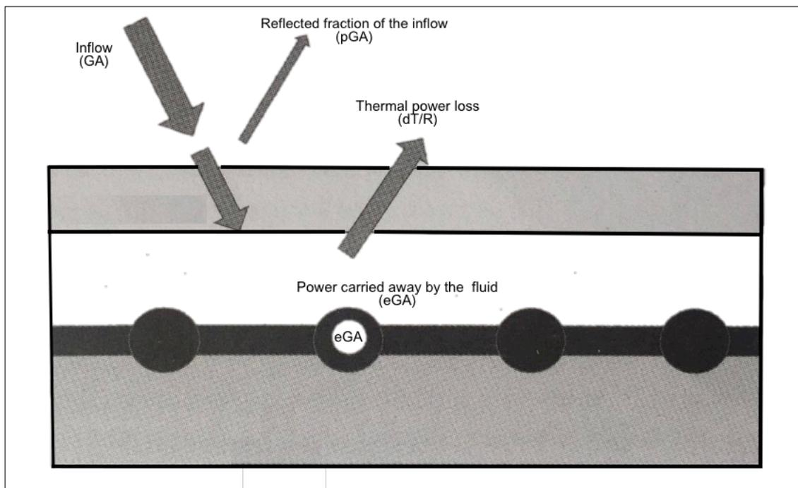
**Figure 29:** Energy flow for a flat-plate solar collector. *Source:* Ehrlich 2013, 286.
