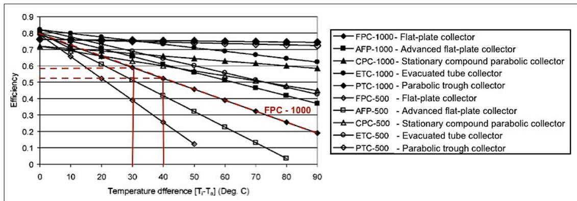
**Figure 30:** Comparison of efficiency of various collectors at two irradiance levels: 500 and 1000W/m<sup>2</sup>. *Source:* Kalogirou 2009, 224.
