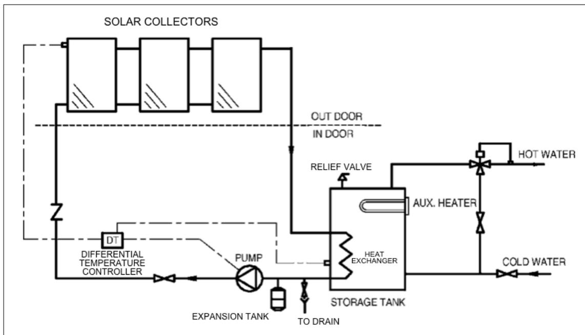
**Figure 26:** Indirect circulation system. *Source:* Kalogirou 2009, 267.
