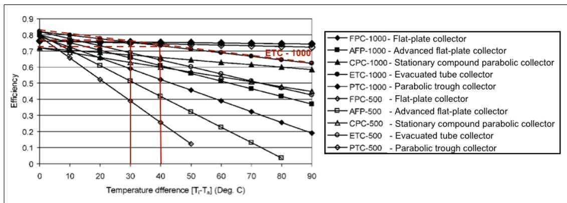
**Figure 31:** Comparison of efficiency of various collectors at two irradiance levels: 500 and  $1000 \text{ W/m}^2$ .
