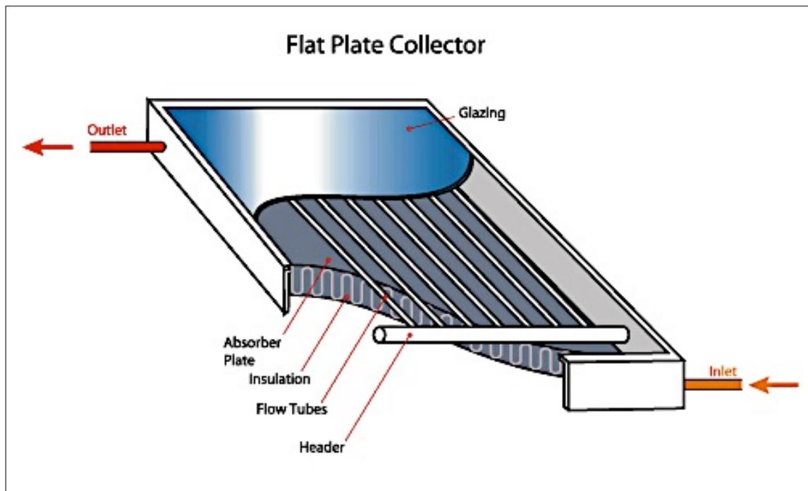
**Figure 19:** A typical flat-plate collector. *Source:* Solar Advice, available from: <https://solaradvice.co.za/flat-plate-solar-water-heating/>
