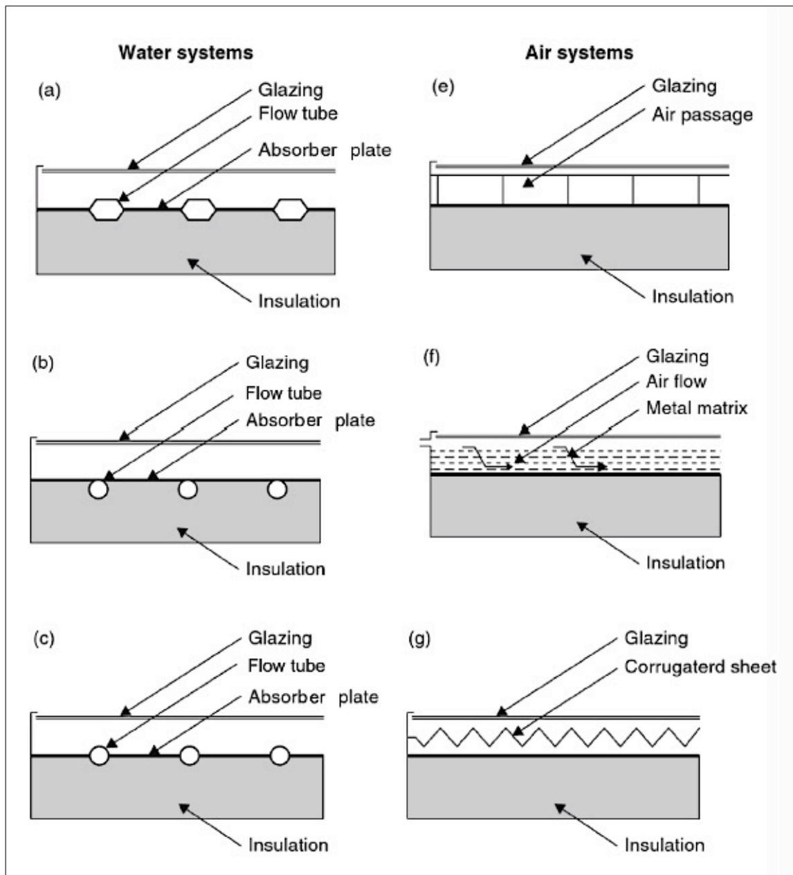
**Figure 20:** Various designs of flat-plate solar collectors for water and air. *Source:* Kalogirou 2009, 128.
