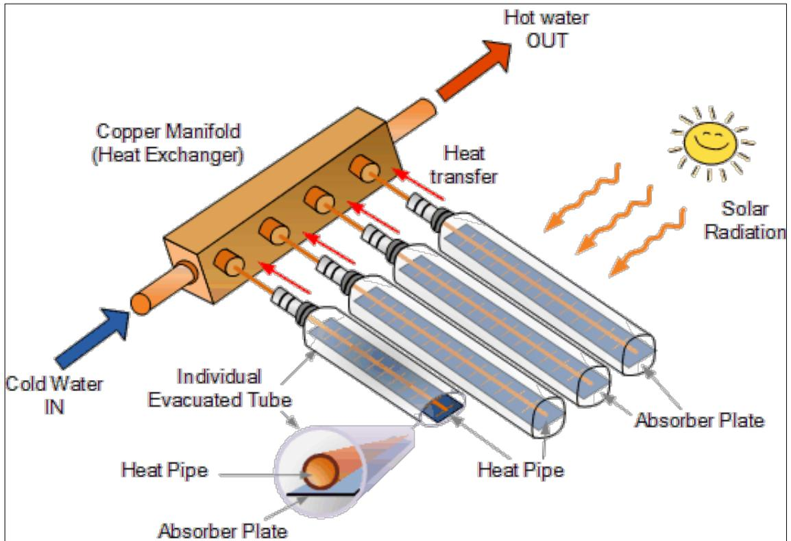
**Figure 21:** Evacuated tube collector. *Source:* Alternative Energy Tutorials, available from: <http://www.alternative-energy-tutorials.com/solar-hot-water/evacuated-tube-collector.html>
