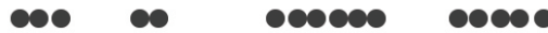
Figure 6.1: Bunched light photon streams. Photons regroup as bunches, which is a manifestation of their bosonic nature [8]
