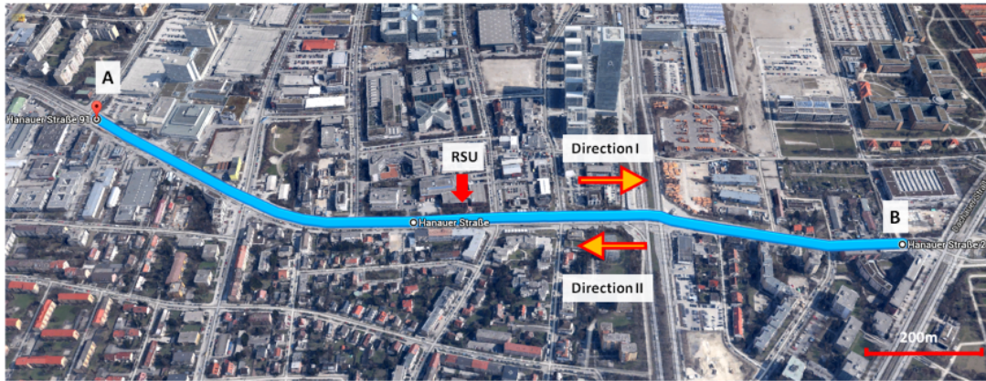
Figure 4.16: Measurement testbed used for 802.11p antenna benchmark.
