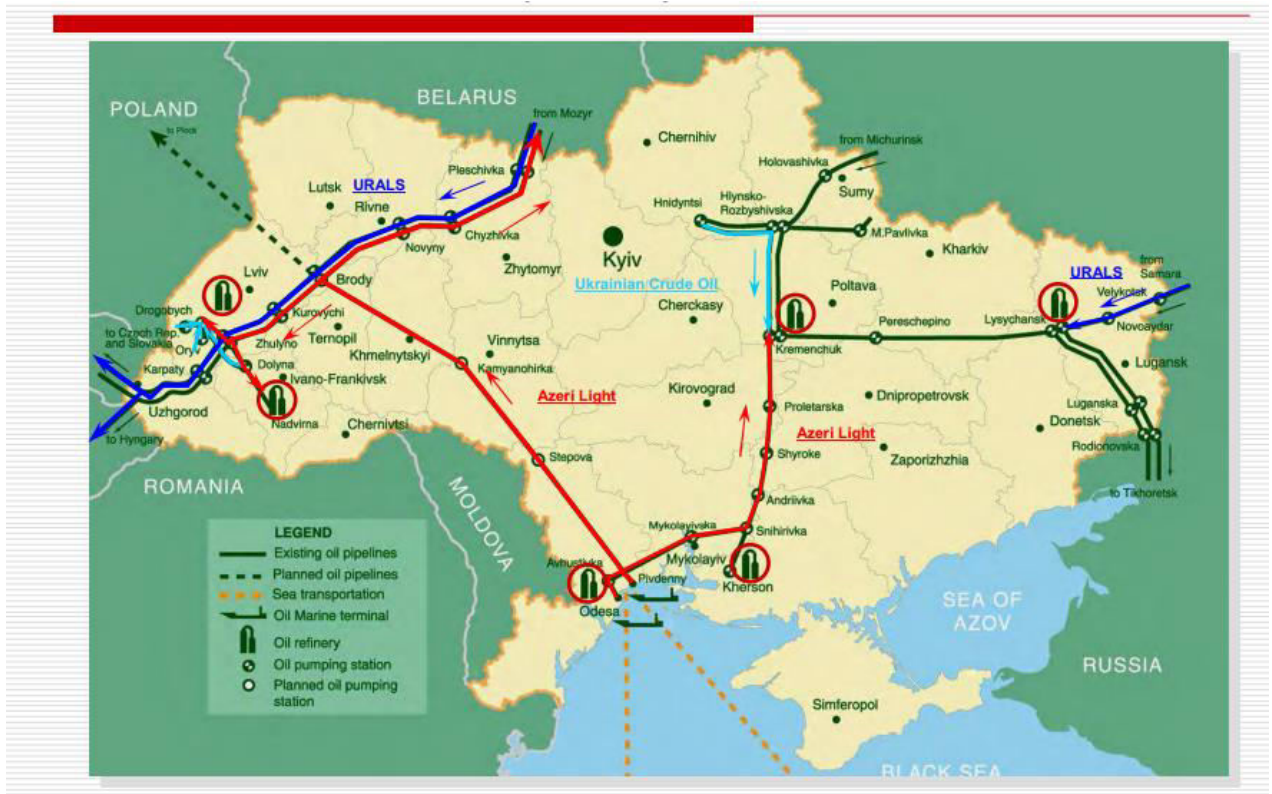
Figure 8. Current routes of oil supplies via oil pipelines
