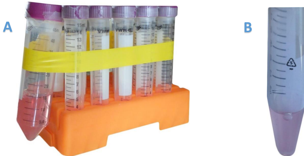
Figure 49: A: Tray with sample tubes (+ 15 ml medium). B: Tube with 1 ml cell suspension
