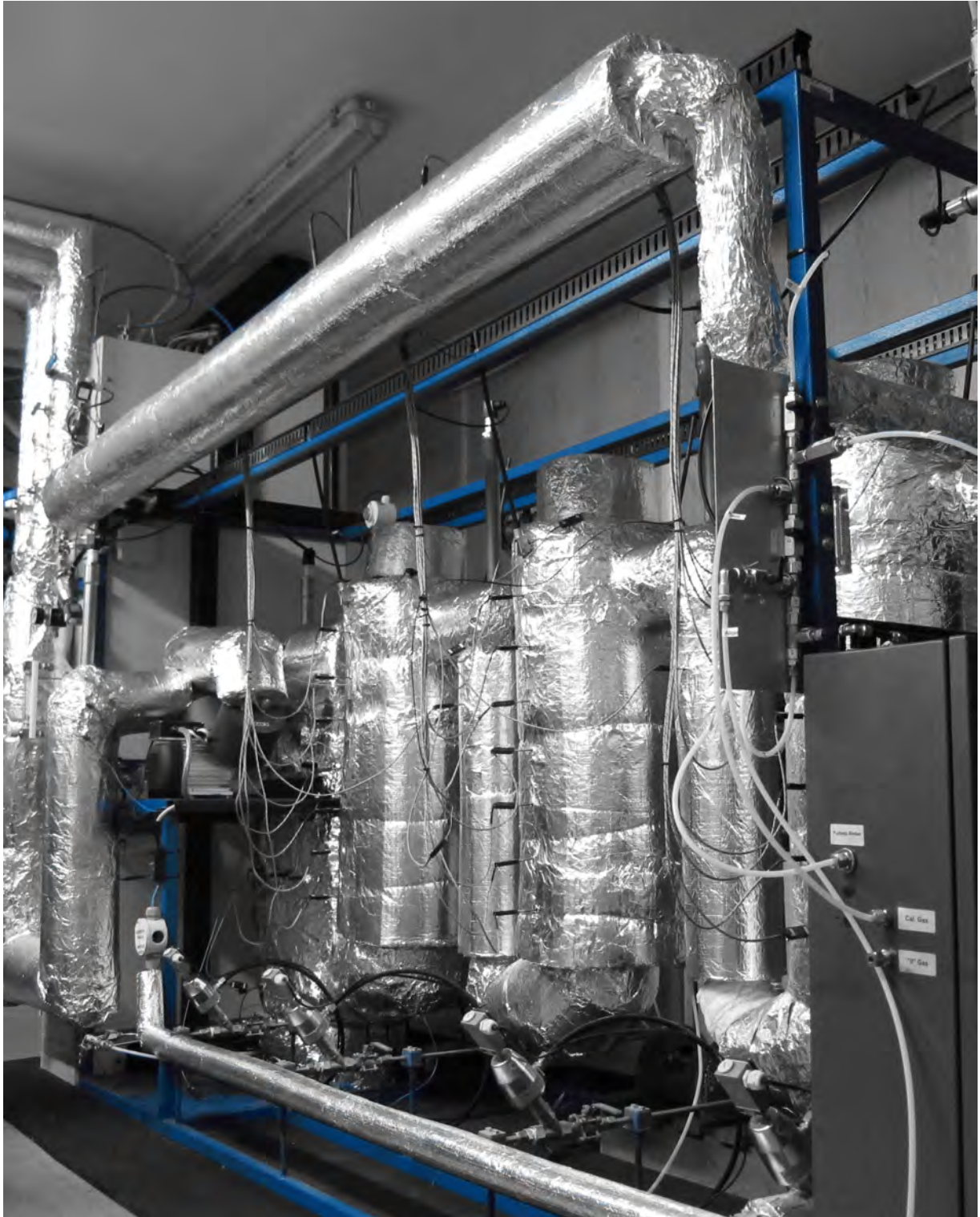
Figure 2: S2 – Picture of the WGS unit employed for fixed bed catalysis of the WGS reaction.
