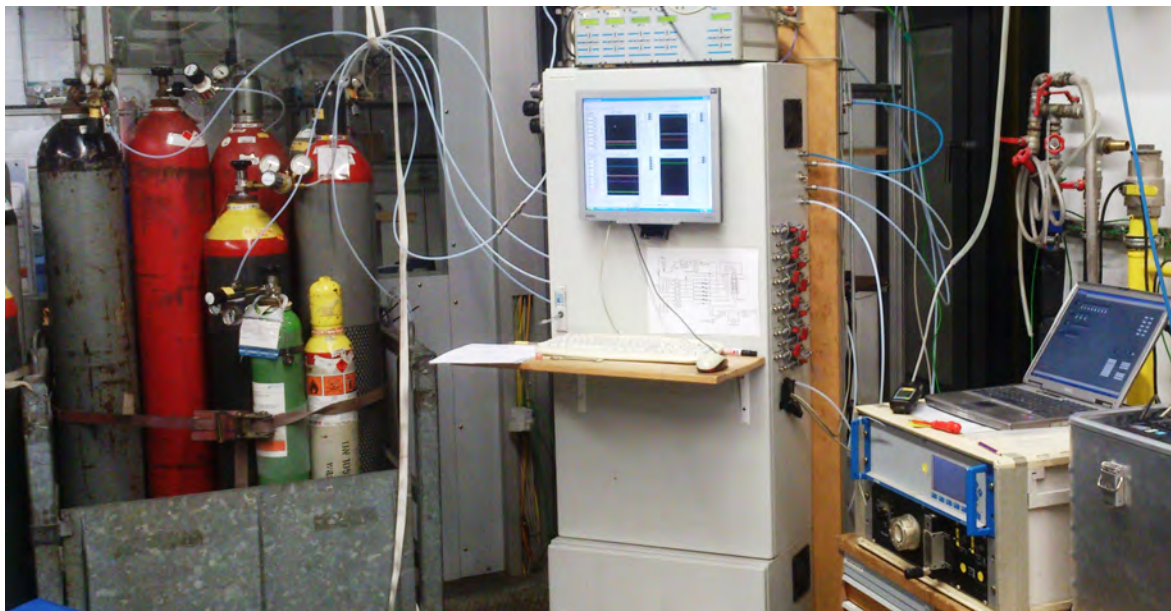
Figure 5.2: Picture of the setup of the "Test rig for chemical kinetics"; left: gas supply with gas cylinders; central: electrical cabinet with mass flow controllers and evaporator, visualization of the experiment, the glass reactor was placed at the backside of the electrical cabinet; right: gas analyzer.
