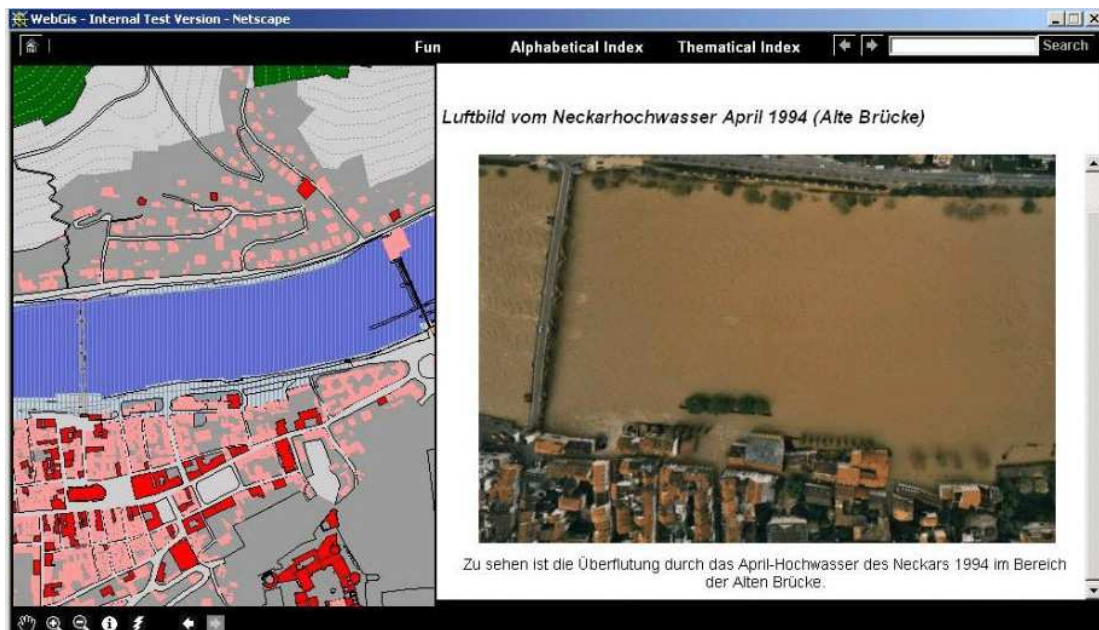
Fig.1: Flood information in the Deep Map WebGIS – the flooded area of the Neckar in Heidelberg April 1994 (stripes) is presented as map layer, right hand the according aerial photo.
