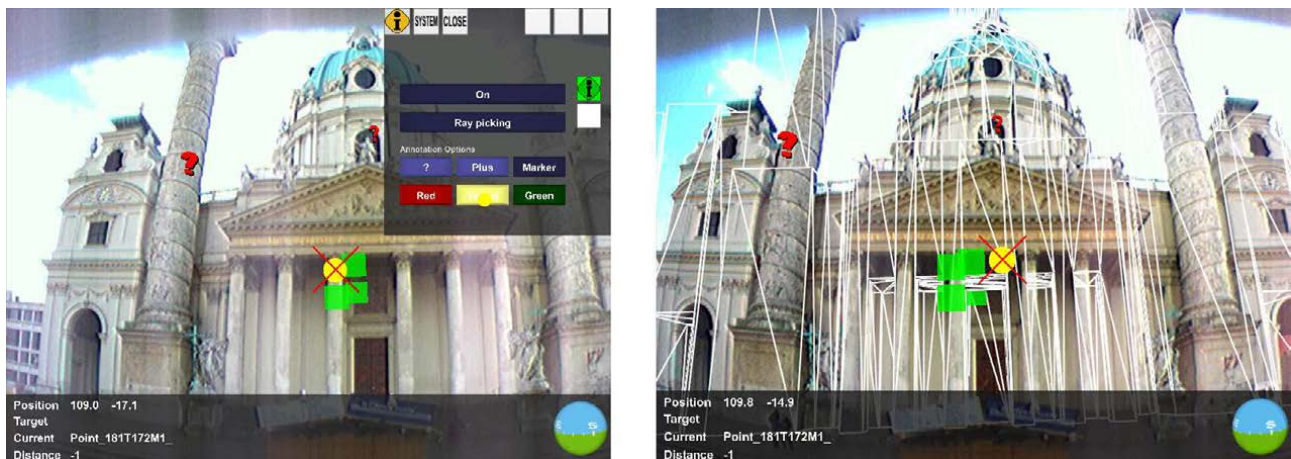
Fig. 5: a) Annotation options and icons. b) The building geometry used for ray intersection is overlaid.
