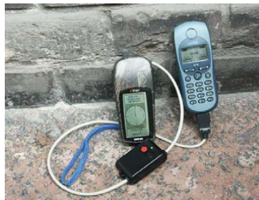
Fig. 4: Mobile phone, GPS and controller units
