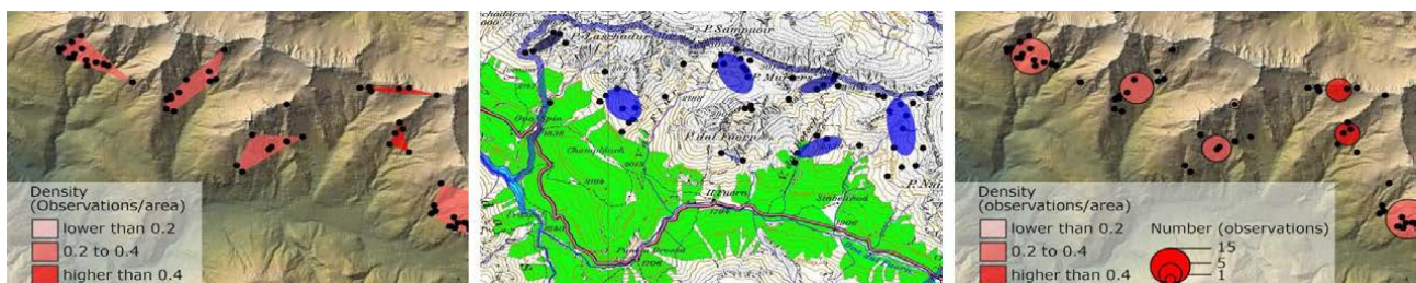
a. Convex hull for detected cluster b. Ellipses with standard deviation c. Count proportional circles Fig. 6: Point generalisation with clustering methods
