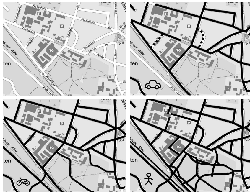
Fig.1: Graphs for route processing depending on moving mode (by car, by bicycle, on foot)
