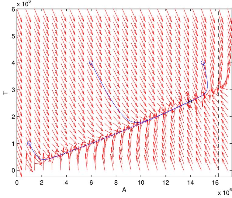
Figure 3.5.: Plot of the phase portrait with parameters  $a = 16250000$ ,  $\alpha = 0.8 \times 10^{-8}$ ,  $\delta = 0.11$ ,  $\beta = 0.5$ ,  $\rho = 0.1$  and some trajectories.
