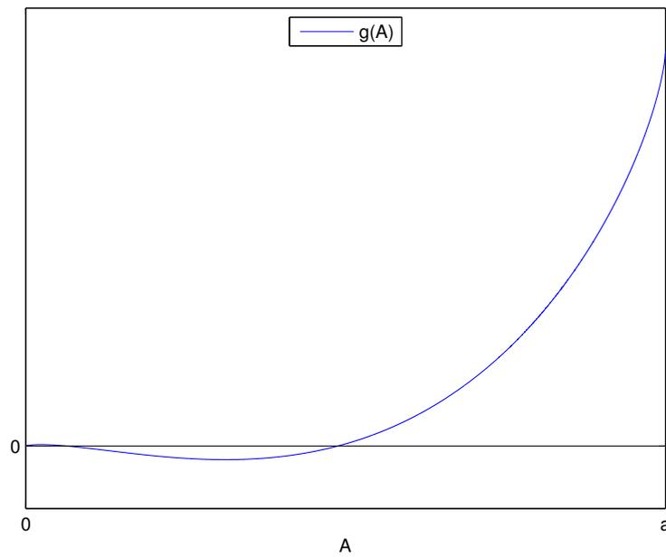
Figure 3.7.: Plot of  $g(A)$  with parameters  $a = 7, \alpha = 0.1, \delta = 0.9, \beta = 0.2, \rho = 0.1, \omega = 1.5, \gamma = -0.4, b_1 = 0.3, b_2 = 0.9$ . (3.16) is not satisfied. Two roots at  $A_1 \approx 0.44$  and  $A_2 \approx 3.42$ .
