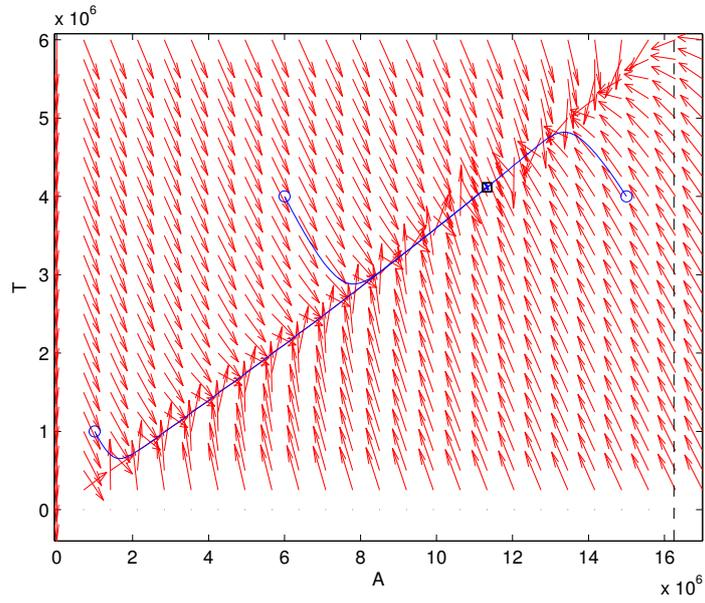
Figure 3.10.: Plot of the phase portrait with parameters  $a = 16250000, \alpha = 1.58 \times 10^{-8}, \delta = 0.2, \beta = 0.2, \rho = 0.1, \omega = 1, \gamma = -0.05, b_1 = 0.05, b_2 = 1$  and some trajectories.
