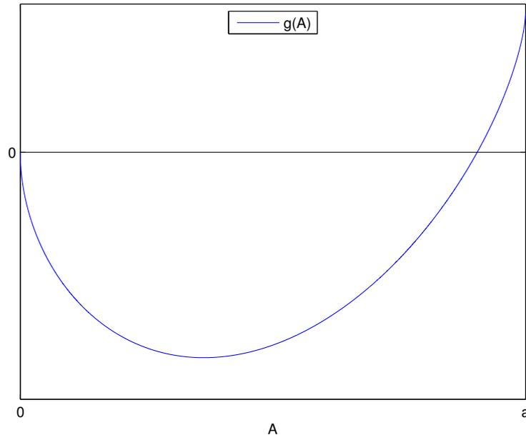
Figure 3.6.: Plot of  $g(A)$  with parameters  $a = 7, \alpha = 0.1, \delta = 0.2, \beta = 0.7, \rho = 0.2, \omega = 0.5, \gamma = -0.4, b_1 = 0.3, b_2 = 0.9$ . (3.16) is satisfied. One root at  $A \approx 6.33$ .
