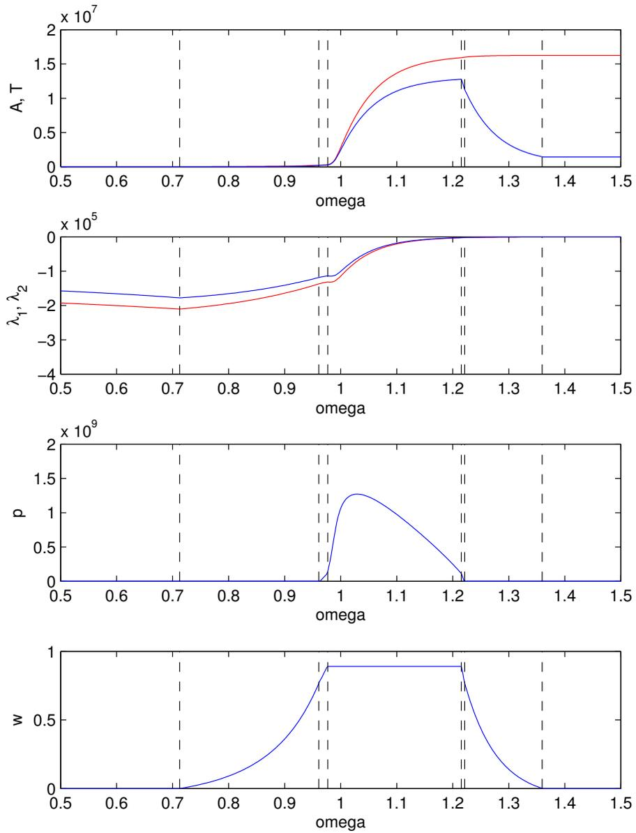
Figure 5.12.: The dashed lines at 0.712, 0.961, 0.977, 1.215, 1.221, 1.360 mark the parameter values where control constraints become active or inactive.  $A$  and  $\lambda_1$  are red.  $T$  and  $\lambda_2$  are blue.
