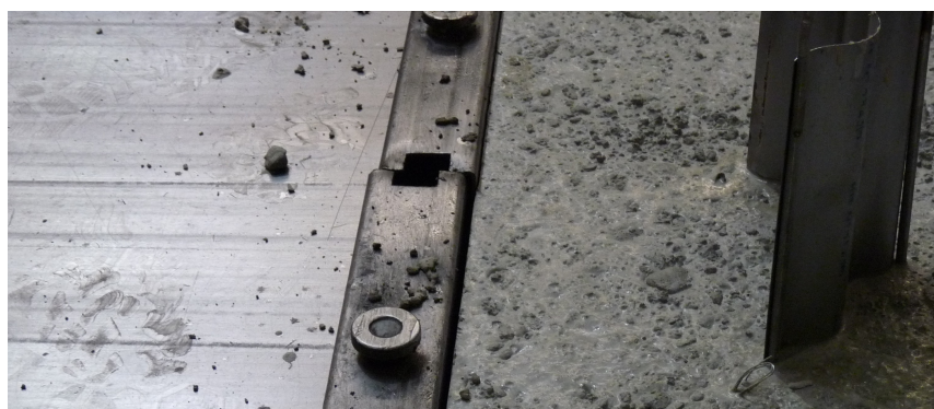
Figure 3.56: The weak formwork fixing magnets cause manufacture errors in the element's outer shape
