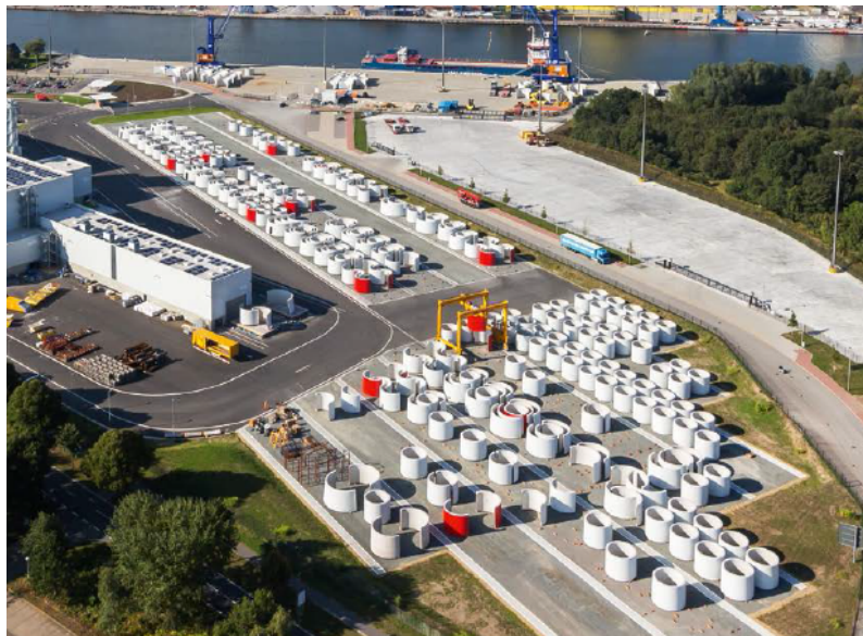
Figure 2.8: Max Bögl's production plant full with precast ring segments for wind turbines at the storage site near the coast in Osterrönfeld, Germany, taken from Max Bögl (2012)
