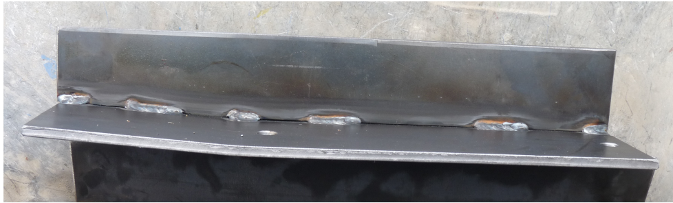
Figure 3.43: Side view of the "T"-shaped steel parts showing the 1.5^\circ bending of the steel which will guide the upper segment
