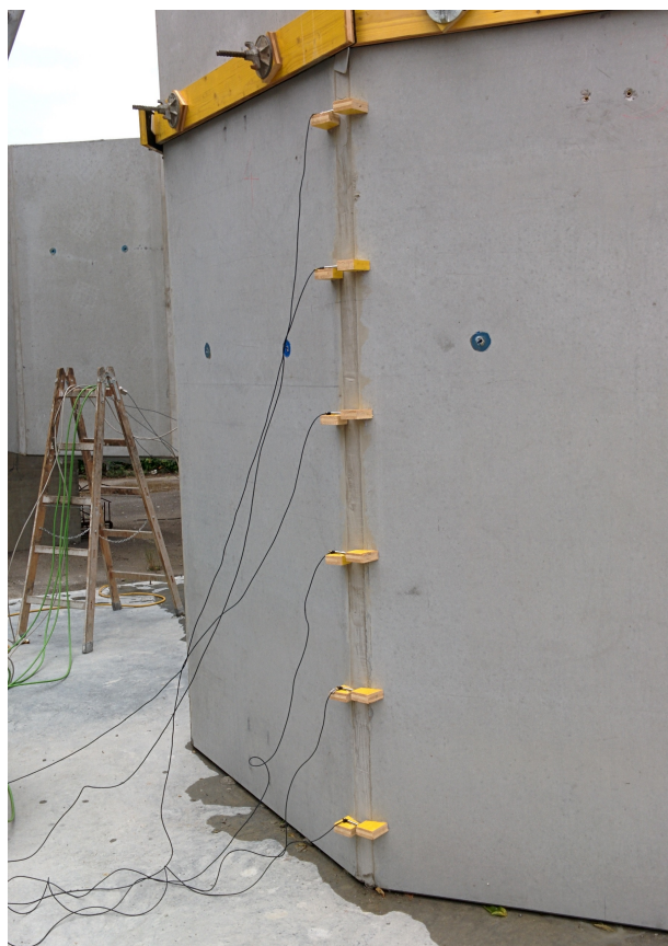
Figure 3.63: The position of the LVDT sensors on the vertical joint between elements 3 and 4
