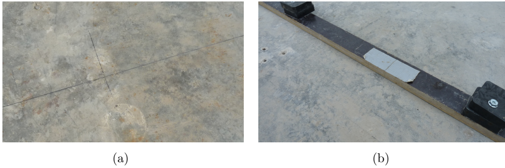
Figure 3.14: Marked polygon sides with (a) the mark for the polygon side midpoint and (b) the planks attached to the polygon sides
