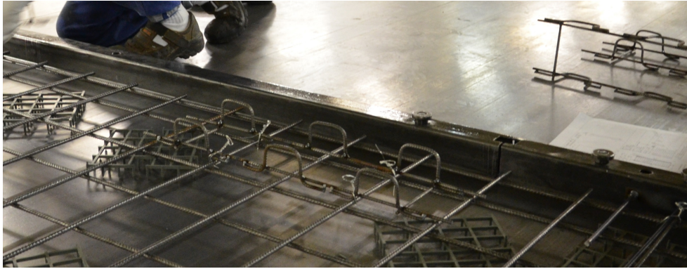
Figure 3.9: Reinforcement loops allow to attach flexible reinforcement in two vertical segment joints
