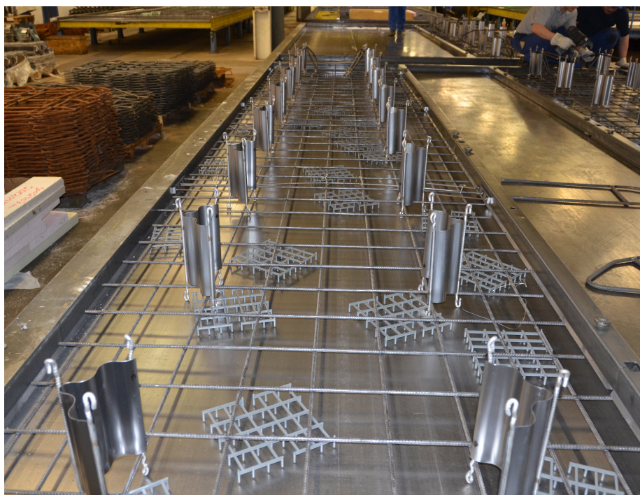
Figure 3.60: Kappema elements - standing on pallet - that are responsible for the interconnection of the shells and the thickness of the element
