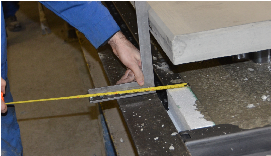
Figure 3.59: Measuring the offset of the elements at the production line while the lower slab is filled with not yet hardened concrete
