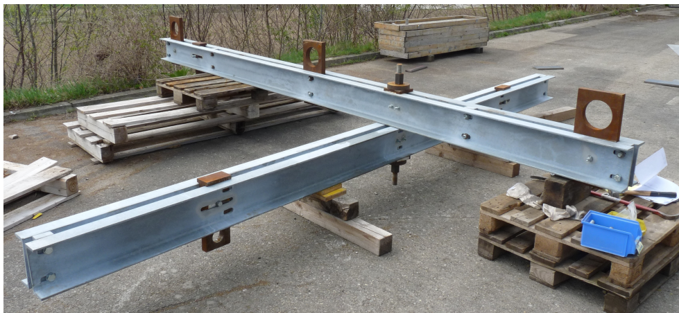
Figure 3.28: The finished spreader, with all connections and lifting steel plates
