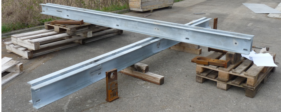
Figure 3.27: Assembly of the spreader, using four U220 profiles
