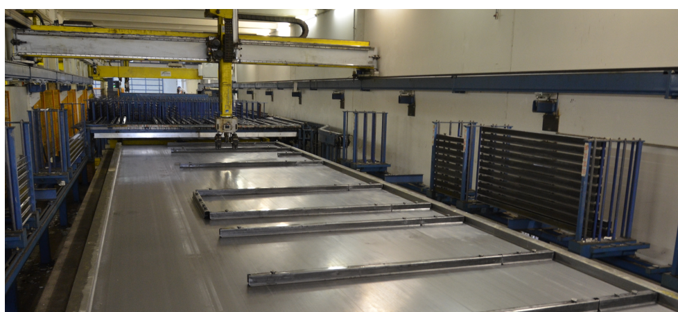
Figure 3.3: Robot in the second station of the double wall production circulation, fixing lateral formwork onto a pallet
