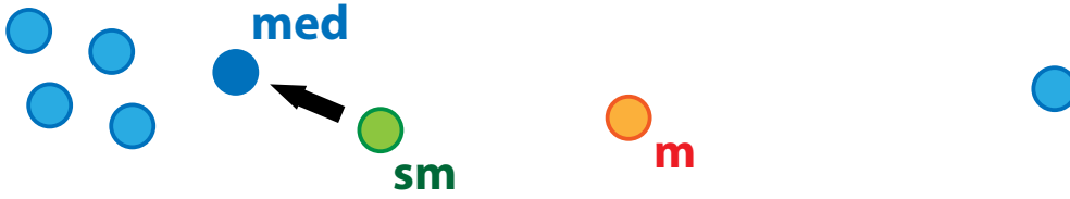
Figure 4.4: Ensemble medoid. The input volumes can be interpreted as points in a k -dimensional space ( blue ). The mean ( m ) is usually prone to follow outliers in the dataset, and the nearest neighbor ( arrow ) of the mean would not be a good representative of the dataset in this case. The spatial median ( sm ) minimizes the Euclidean distances to all points, but is generally not a part of the dataset. We therefore find the point that is closest to the spatial median ( arrow ) and use this as the medoid ( med ) of the ensemble.
