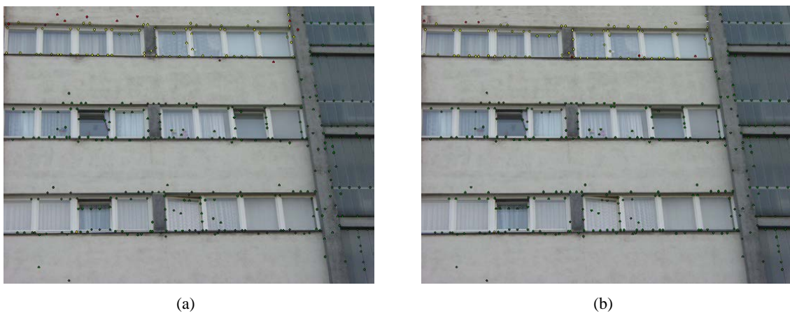
Figure 7.2: (a) Points detected by the Förstner 2 operator; (b) matched points.
