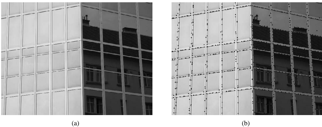
Figure 6.11: (a) Image with strong reflections on the right side; (b) interest points detected with the Förstner 2 and the Harris operator.
