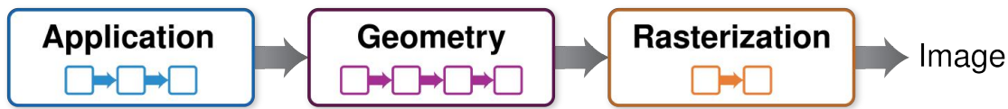
Figure 1.1: The basic rendering pipeline. This pipeline is composed of three conceptual steps: application, geometry and rasterization. These stages can be parallelized and can be pipelines themselves. The pipeline model is adopted by modern graphics hardware. This allows the GPU to parallelize operations in several pipeline stages.
