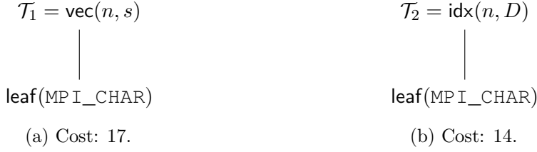
Figure 7.5: Two type path representations for a type map M = (\langle \text{char}, \dots \rangle, \langle 0, s, 2s, \dots \rangle) of arbitrary length n . For Träff’s type path normalization algorithm [Trä14], the representation \mathcal{P}_1 given in Figure 7.5a constitutes the best case, whereas the representation \mathcal{P}_2 from Figure 7.5b constitutes the worst case. A type path of height d with the longest occurring displacement sequence being of length l is normalized in O(dl\sqrt{l} + (d \log l)^3) time. The representation \mathcal{P}_1 does not contain any displacement sequence and the depth is constant w.r.t. n . It can thus be normalized in constant time. The algorithm, however, requires O(n\sqrt{n}) time to normalize the representation \mathcal{P}_2 , since the longest occurring displacement sequence is of length n . Our approach, which is to flatten the input type path and perform type path reconstruction on the resulting type map, requires O(n \log n / \log \log n) time in both cases. Flattening the type paths \mathcal{P}_1 and \mathcal{P}_2 can trivially be done in O(n) time. Our approach is thus asymptotically faster for the representation \mathcal{P}_2 , but slower for the representation \mathcal{P}_1 .
