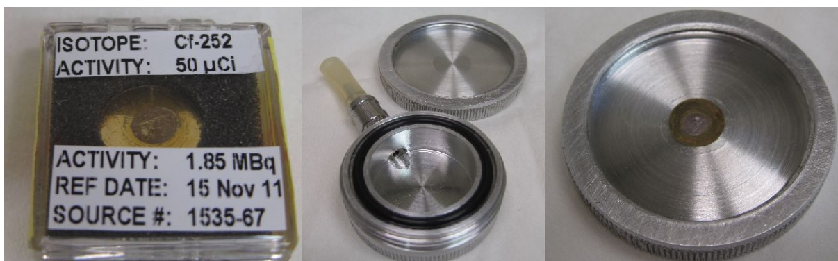
Figure 5.1: Left: The ^{252}\text{Cf} foil in its original container. Middle: The AXG1 aluminium container with the connector valve. Right: The ^{252}\text{Cf} foil glued onto the cap of the AXG1.
