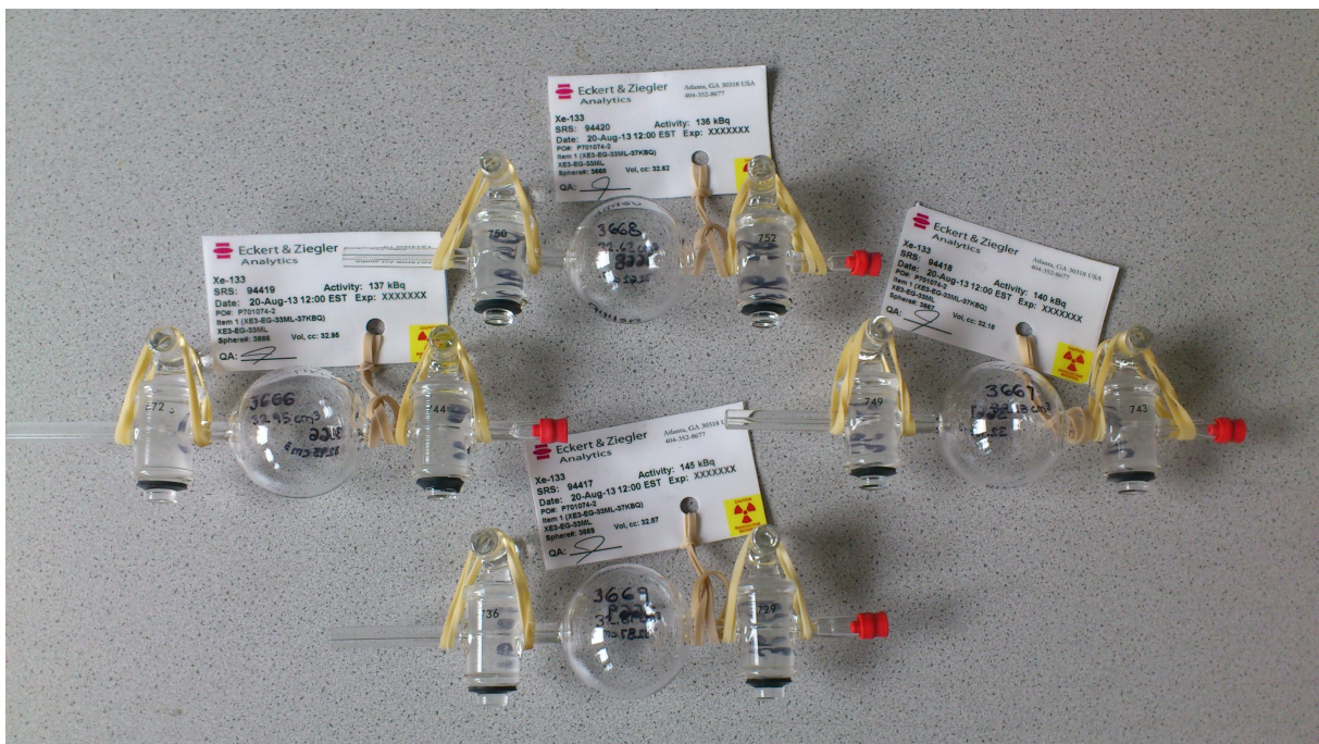
Figure 5.8: Four ^{133}\text{Xe} standards as they are supplied by Eckert & Ziegler / Analytics.
