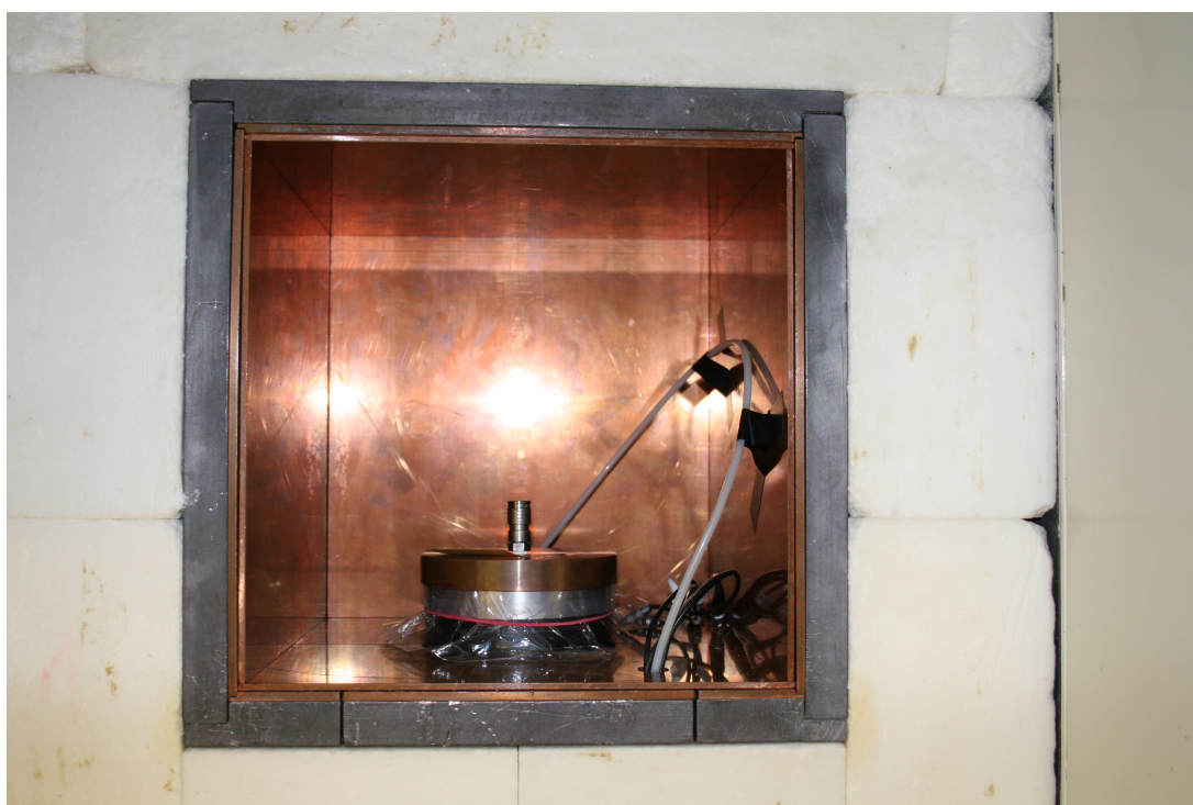
Figure 3.9: A radioxenon measurement cell on the detector Det4.
