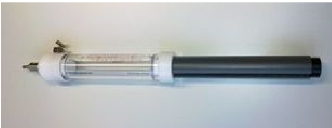
Figure 3.7: The gas-tight syringe and the plunger holder.
