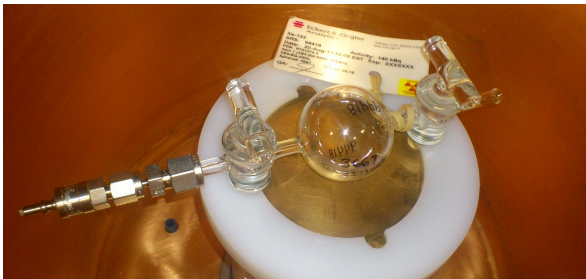
Figure 5.9: A ^{133}\text{Xe} standard with a connector valve mounted on detector Det3.
