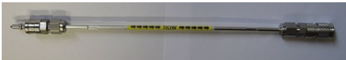
Figure 5.2: The filter tube used for separation of particulate and aerosol-bound fission products from noble gases.
