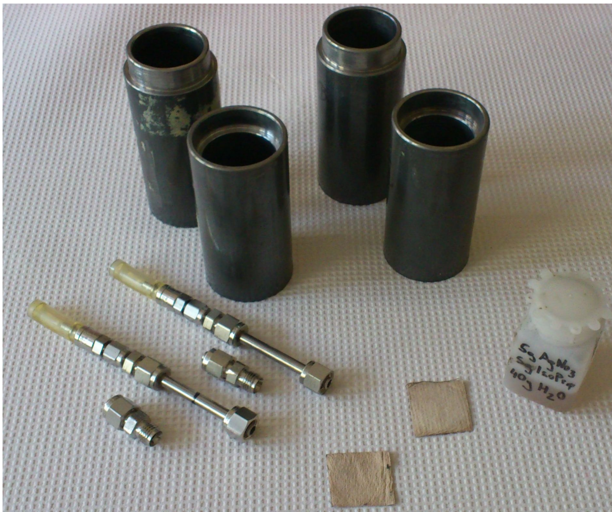
Figure 5.6: The AXG2 work desk: two open generators with two Petri filter sheets, the silver nitrate solution and the lead shieldings for transport.
