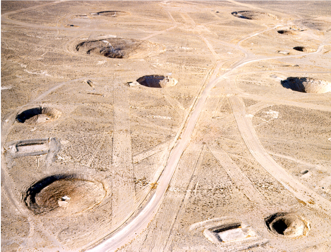
Figure 1.1: Subsidence craters, caused by underground nuclear explosions in the Nevada test site.
