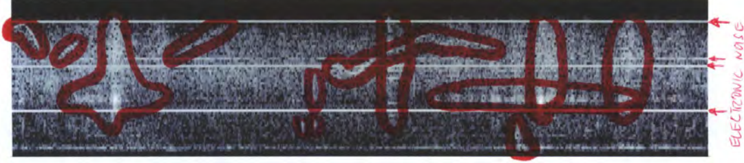
Figure 5.2: Simple detection of event patterns using a printout and a pen. For humans it is very easy to quickly outline connected patterns in the spectrogram, even if they are overlapping. With some background knowledge and experience characteristic events can also be classified (e.g. electronic noise).
