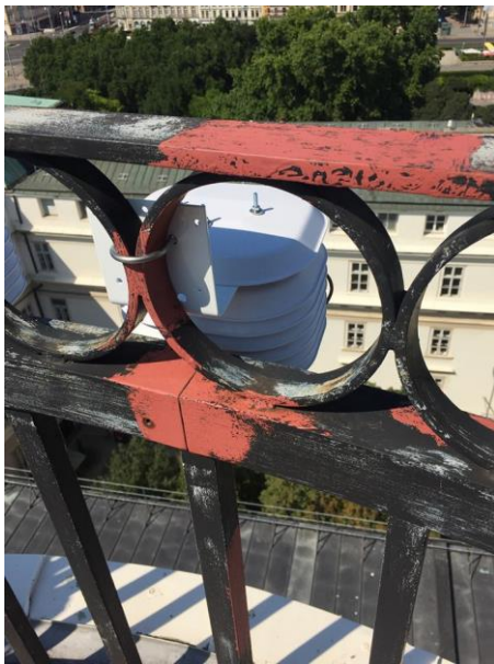
Figure 7: Temperature and humidity sensor fixed on balcony railing
