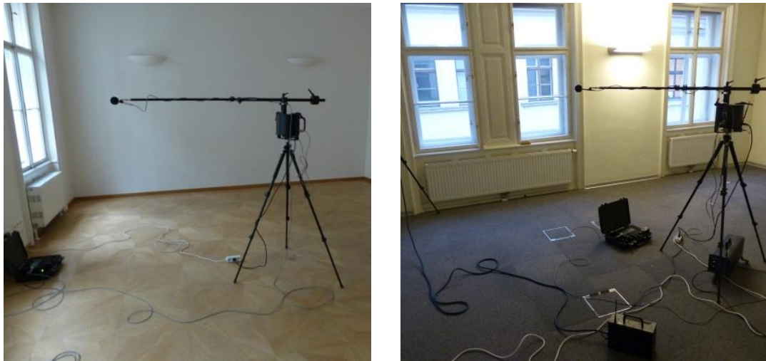
Figure 10. Receiving room (left);Source room (right)
