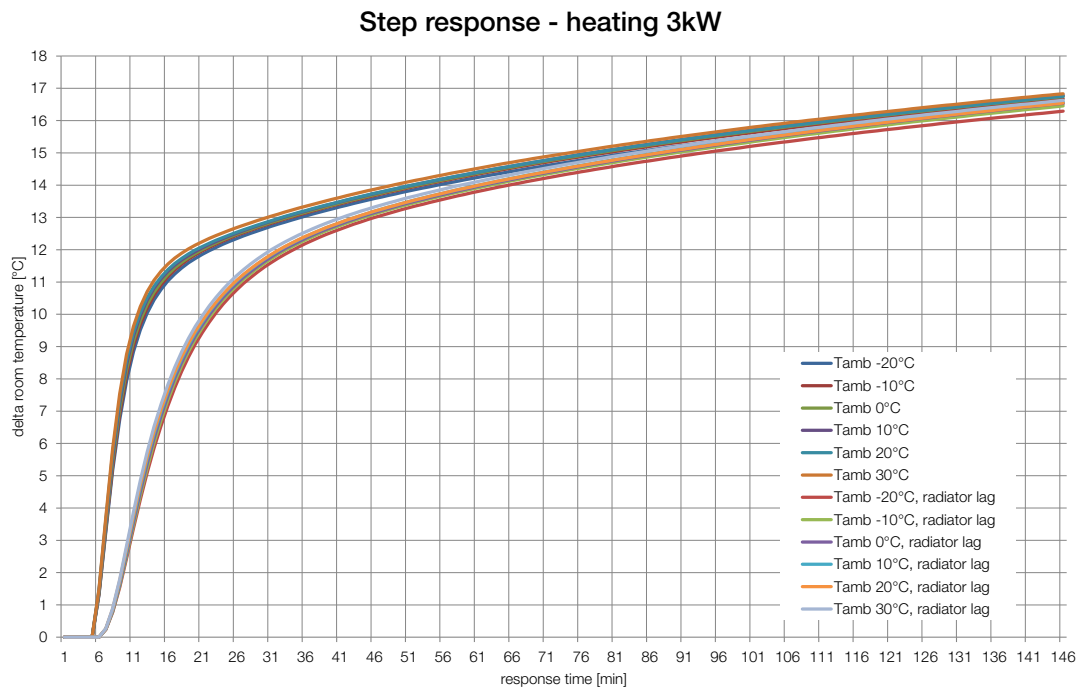
Figure 6.3 - step response wo/w radiator lag
