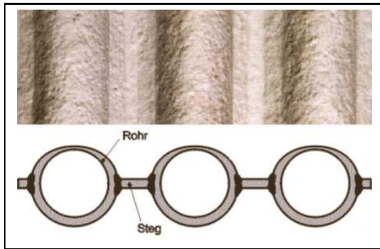
**Figure 3.2.:** One Side Heated Membrane Wall, Tube - Fin - Tube [6]
