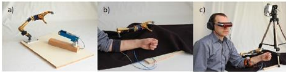
Figure 50: The experimental setup for the study of prosthesis closed loop control: a) sensor hand speed and the dynamometer, b) the myoelectric interface to the prosthesis, and c) the complete setup including the haptic device and the video system.
