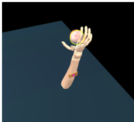
Figure 71: A virtual-reality scenario implemented to evaluate the level of Performance_1. The subjects have to move only the elbow back and forth between the object and release position.
