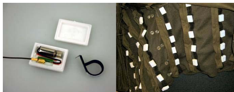
Figure 11: TNO custom rotary-inertial tactor (left). TNO tactor array housed in vest (right) (Mcgrath et al. 2008)
