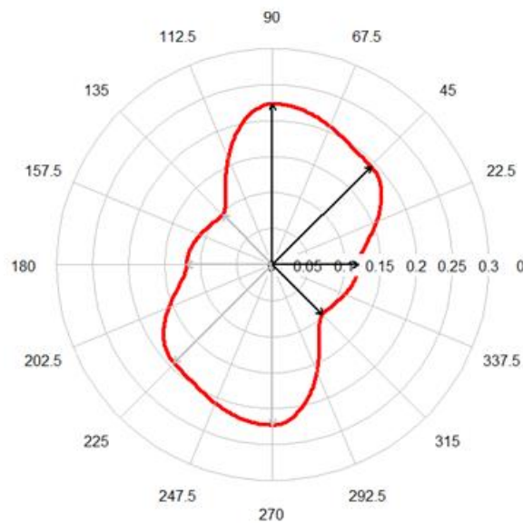
Figure 45: The fitted Weber Function was obtained interpolating pairs of measured WFs (black/gray arrows) by a spline (the red profile).
