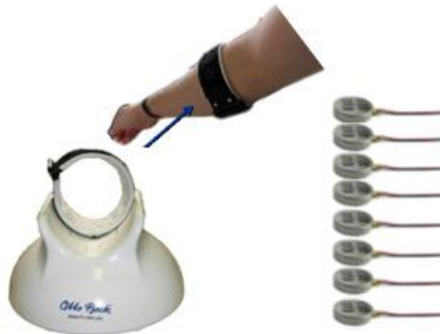
Figure 18: A linear array comprising eight vibration motors. The motors were activated in sequences aiming to induce sensation of movement in the subjects' forearm, correspondent with the prosthesis movement, or were simultaneously activated in static patterns to transmit grasp force.
