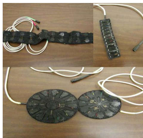
Figure 9: Examples of rubber array electrodes used for electro-stimulation (McGrath et al. 2008)
