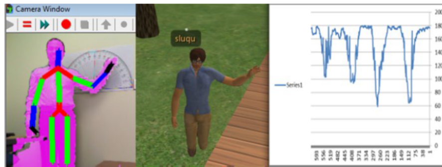
Figure 2.6: Second Life virtual environment (center) being mapped to physical environment (lef) with the graph of the angle at the elbow produced by moving the arm (right) [1].
