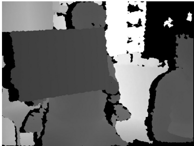
Figure 4.2: Depth image produced by Kinect sensor [72].
