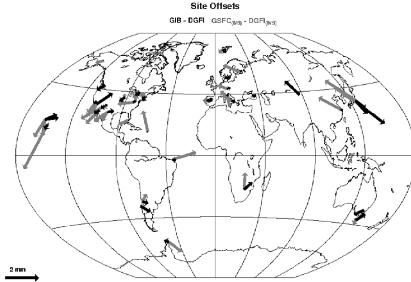
Figure 4. Horizontal offsets of all VLBI stations, GIB - DGFI differences in black, GSFC IVS and DGFI IVS differences in grey
