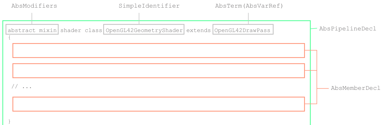
Figure 5.5: A shader declaration with according modifiers and a class name. After the extends keyword there is a list of terms denoting the base classes. Inside the shader scope several member definitions can be found.
