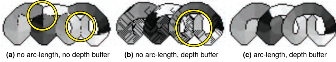
Figure 2.5: Comparison when using the arc-length parametrization or depth buffering for visibility. Since the grayscale gradients are stored in the data, they should be clearly reflected in the lumen visualization. Artifacts (highlighted with yellow circles) occur in (a) because pixels are never changed and in (b) since too many pixels are falsely overwritten. (c) shows the result of our proposed method.
