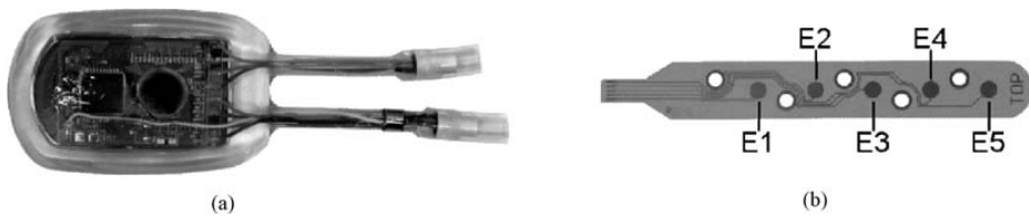
Fig. 1. Components of the implantable EMG measurement system: (a) Central implant (size: 38 \times 25 \times 8 mm) consisting of electronics capsuled in silicone (Center for Medical Physics and Biomedical Engineering, Medical University of Vienna). (b) Polyimide thin film electrode array (size: 28 \times 3 \times 0.02 mm). Dark circles are contacts surfaces (E1–E5), white circles are suture holes for electrode fixation.
