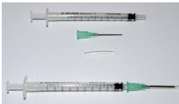
Figure 4.8: A 1 mL syringe, a 0.8 mm cannula and a piece of rubber tube (top) that were combined (bottom) to create a tool for administering the particle solutions to the microfluidic channel
