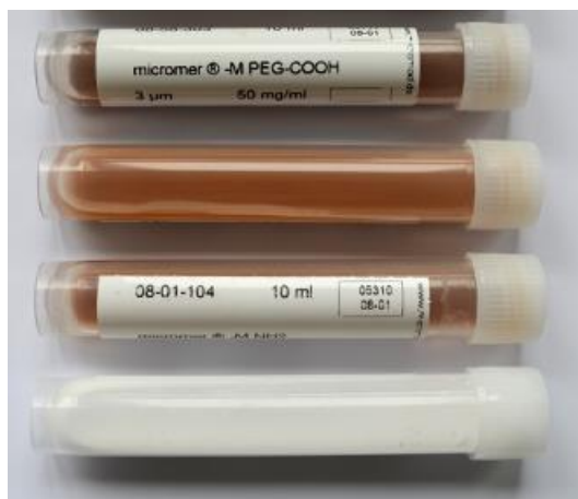
Figure 4.7: Magnetic particles (three tubes on top with brown content) and non-magnetic particles (tube on bottom with white content) purchased from micromod Partikeltechnologie GmbH
